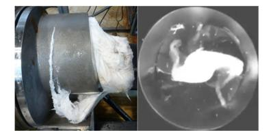
**Figure 11.** Modification 1—clogging after long-time functional test (BEP, L25) (**left**) and optical investigations (**right**).
