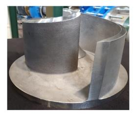
Figure 4. Modification 0-manufactured impeller.
