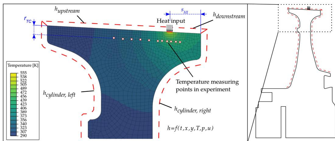
Figure 2. Two-dimensional finite element model [7].
