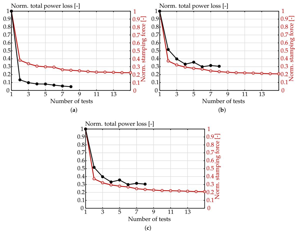
**Figure 14.** Normalised total power loss at the beginning of the rub test (●) and normalised stamping force (○). (a) Seal O and rotor–seal interference of 0.1 mm, (b) seal O and rotor–seal interference of 0.2 mm, (c) seal S and rotor–seal interference of 0.3 mm.
