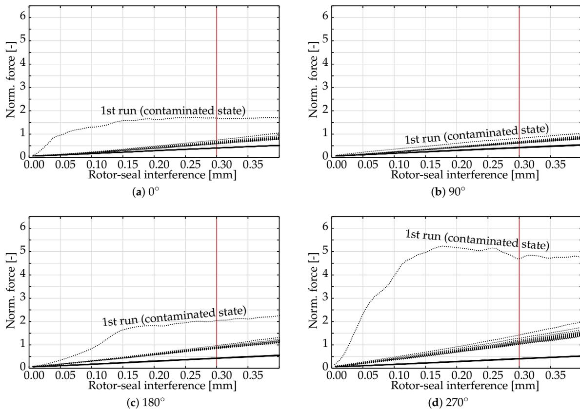
**Figure 5.** Normalised stamping force over rotor–seal interference for seal *S* at four circumferential positions before (—) and after the treatment (•••); the measurements were carried out by MTU Aero Engines AG.
