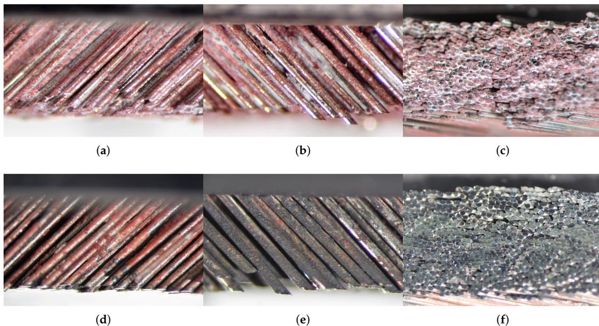
**Figure 9.** (a) Microscope image of seal S front plate side before experiments, (b) microscope image of seal S back plate side before experiments, (c) microscope image of the underside of bristle package of seal S before experiments, (d) microscope image of seal S front plate side after experiments, (e) microscope image of seal S back plate side after experiments, (f) microscope image of the underside of bristle package of seal S after experiments.
