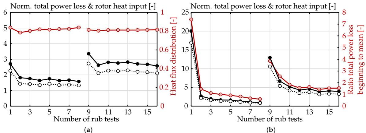
**Figure 10.** (a) Normalised total power loss (●—), rotor heat input (●··) and heat flux distribution (—●); the results shown represent values averaged over the rubbing duration. (b) Normalised total power loss (●—), rotor heat input (●··) and ratio of total power loss at the beginning to averaged value (—●); the shown power losses and heat inputs represent values at the beginning of the rubbing duration.
