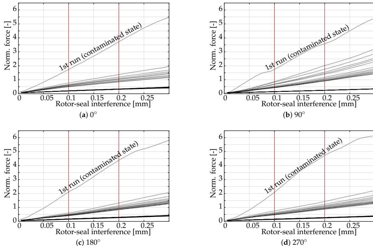
**Figure 4.** Normalised stamping force over rotor–seal interference for seal O at four circumferential positions before (—) and after the treatment (···); the measurements were carried out by MTU Aero Engines AG.
