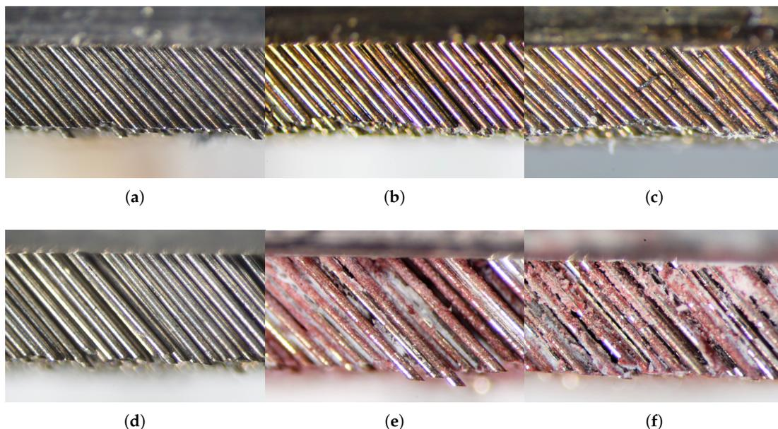
**Figure 3.** (a) Microscope image of seal *O* before treatment, (b) microscope image of seal *O* after treatment, (c) microscope image of seal *O* after stiffness measurement, (d) microscope image of seal *S* before treatment, (e) microscope image of seal *S* after treatment, (f) microscope image of seal *S* after stiffness measurement; the preparation was carried out by Siemens AG and MAN Energy Solutions SE.
