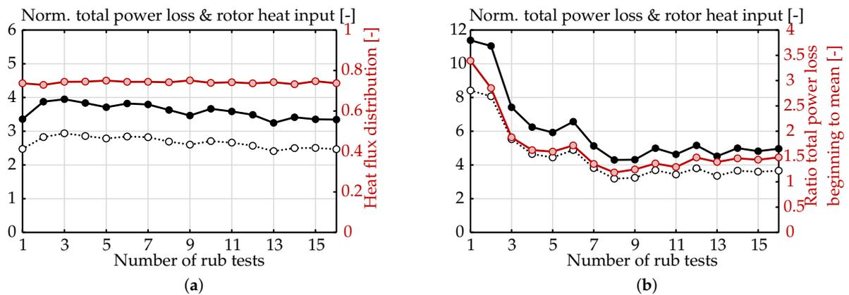
**Figure 6.** (a) Normalised total power loss (—●—), rotor heat input (•○•) and heat flux distribution (—○—); the results shown represent values averaged over the rubbing duration. (b) Normalised total power loss (—●—), rotor heat input (•○•) and ratio of total power loss at the beginning to averaged value (—○—); the shown power losses and heat inputs represent values at the beginning of rubbing.
