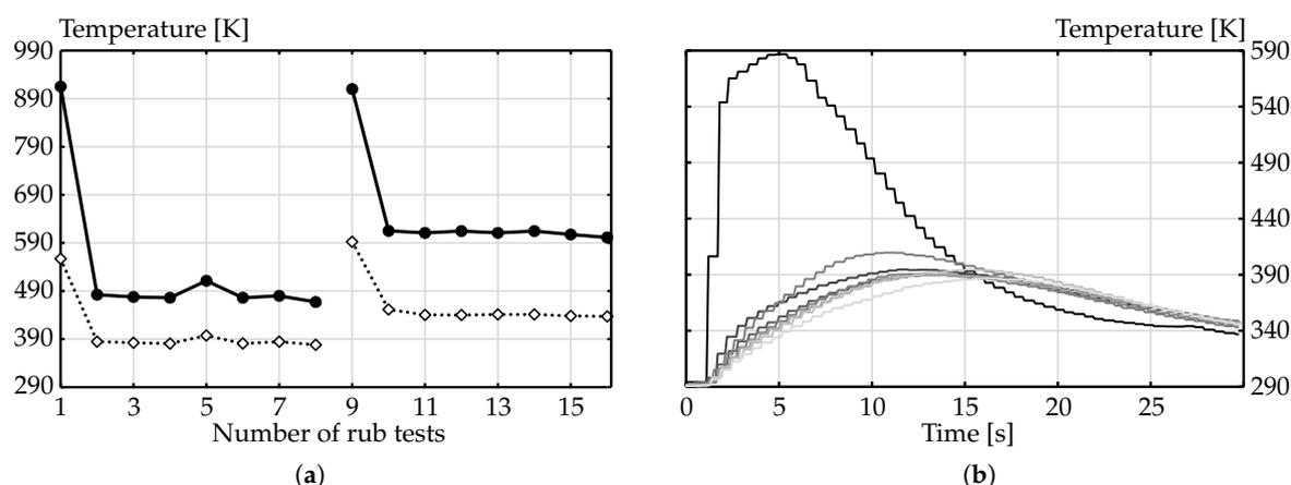
**Figure 11.** (a) Maximum temperature in the contact zone between seal and rotor (value out of FEA) (●) and maximum rotor temperature (◇). (b) Course of the maximum rotor temperature over the rubbing duration, first run (—) to last run (—).
