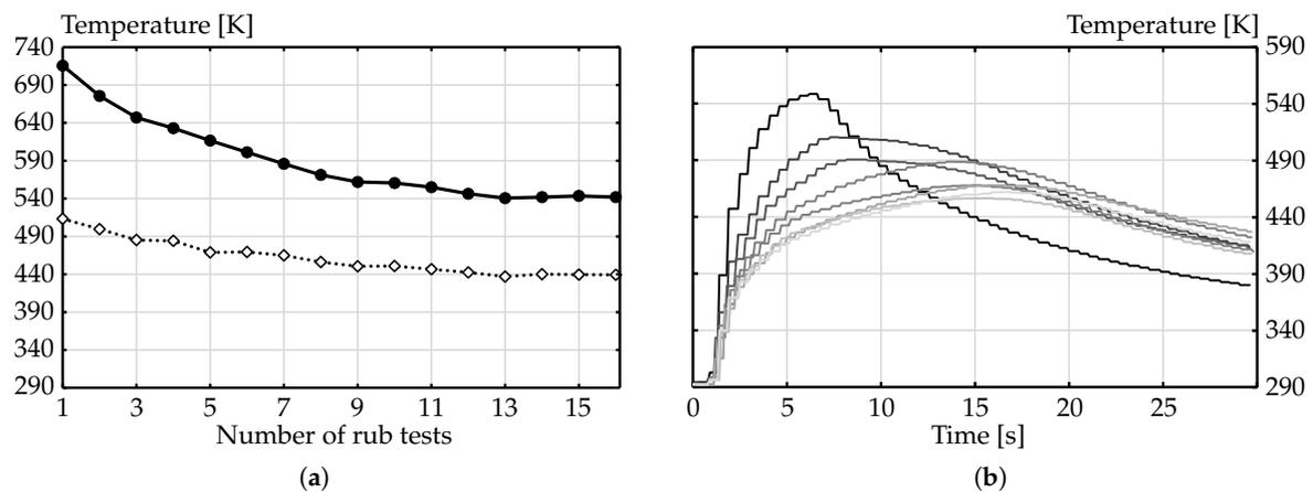
**Figure 7.** (a) Maximum temperature in the contact zone between seal and rotor (value out of FEA) (—●) and maximum rotor temperature (•◇•). (b) Course of the maximum rotor temperature over the rubbing duration, first run (—) to last run (—).
