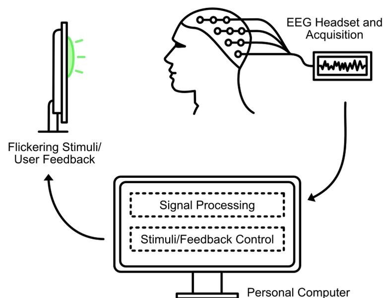
**Figure 1.** General structure of an SSVEP BCI.
