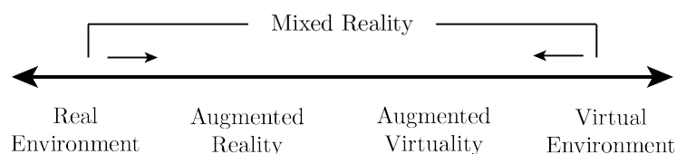
Figure 3. Simplified representation of virtuality continuum (based on the figure proposed by Milgram and Kishino [18]).
