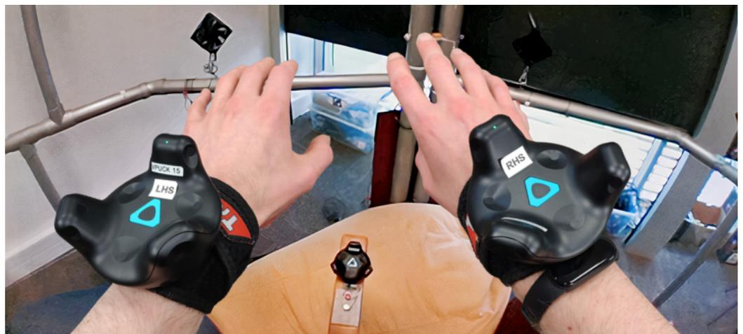
**Figure 9.** An example of how Vive tracker pucks were strapped to each hand.
