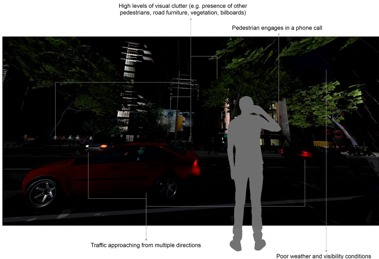
**Figure 10.** “Complex” simulated crossing scenario for eHMI testing. The scenario consists of a road site where traffic approaches from two lanes and joins the main road from side streets, adverse weather and poor visibility conditions, high levels of clutter in the scene as well as the presence of the phone call distraction.
