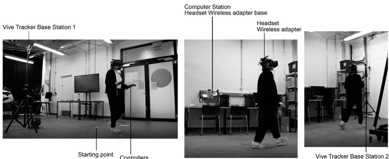
**Figure 5.** Virtual reality setup and walking area. Tracker base stations face each other diagonally, defining the walking area. The VR headset is fitted with a wireless adapter, of which the base is attached to the computer’s monitor, which allows free movement within the walking area.
