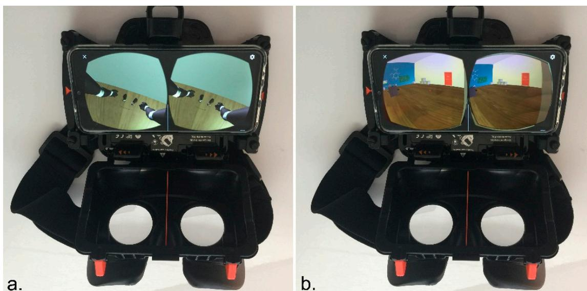
**Figure 1.** Screenshots of the system operating in a smartphone embedded in a head-mounted display (HMD): (a) Image of the user's digital body representation in the virtual reality (VR) environment. (b) Image of the virtual classroom with the hovering molecular structures under investigation.
