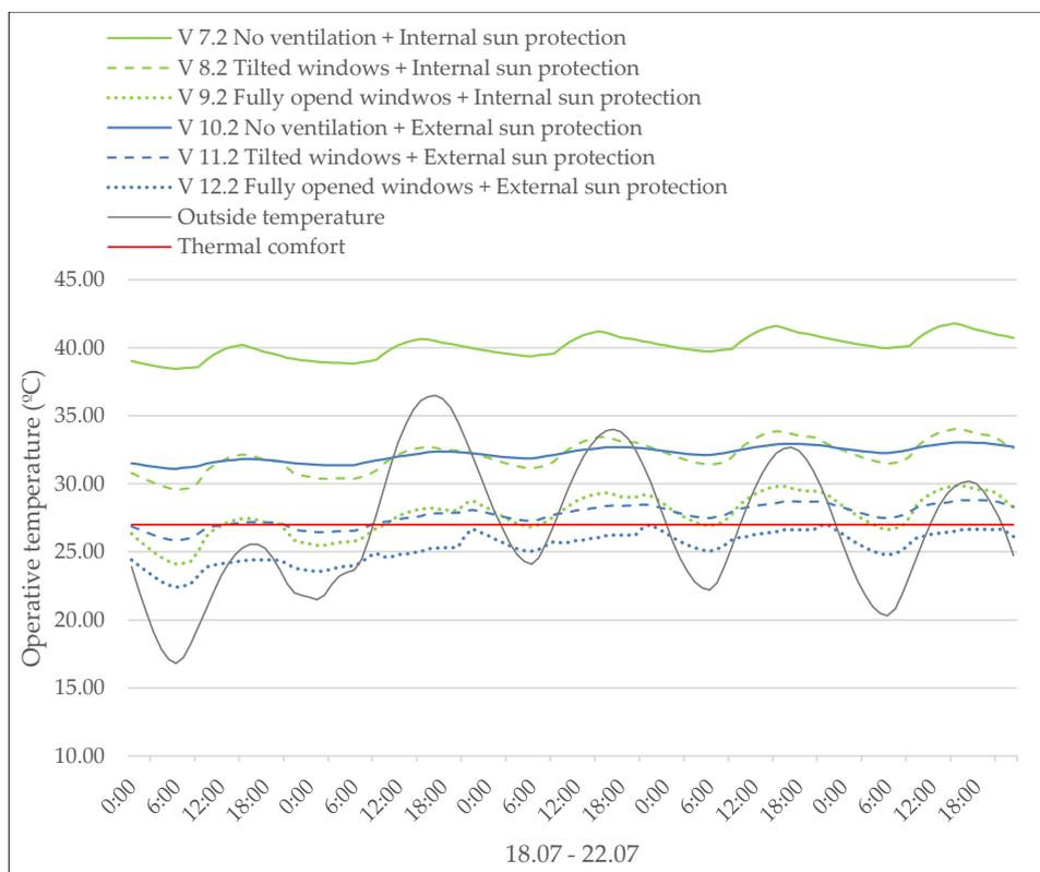
Figure 7. Future climate scenario—Variants of sun protection and night ventilation, based on [33].
