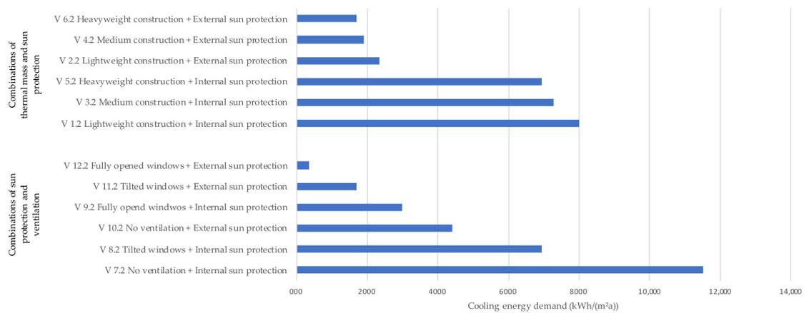
Figure 9. Future climate scenario—Cooling energy demand, based on [33].
