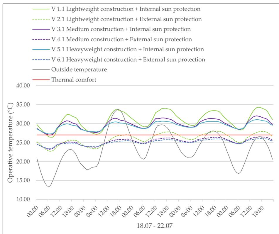
Figure 4. Current climate scenario—Variants of thermal mass and sun protection, based on [33].
