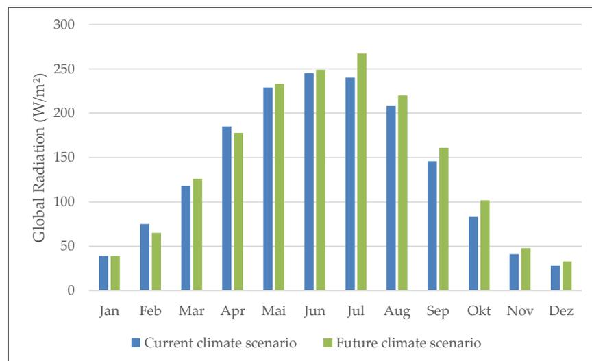
**Figure 3.** Monthly global radiation based on long-term measurements (1991–2010) for the location Wien Hohe Warte [30].
