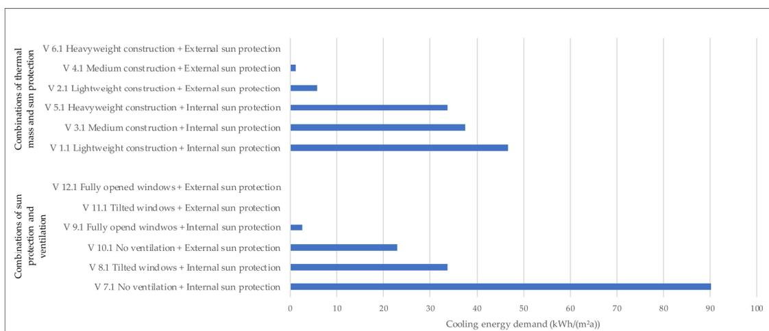
**Figure 8.** Current climate scenario—Cooling energy demand, based on [33].
