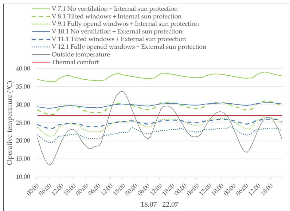
**Figure 5.** Current climate scenario—Variants of sun protection and night ventilation, based on [33].
