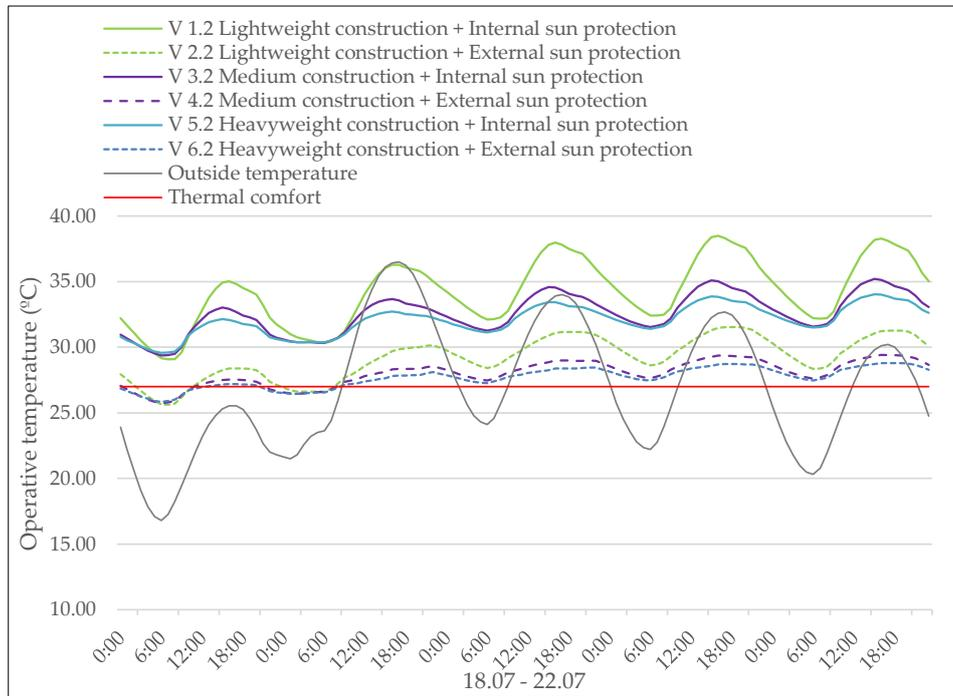
Figure 6. Future climate scenario—Variants of thermal mass and sun protection, based on [33].
