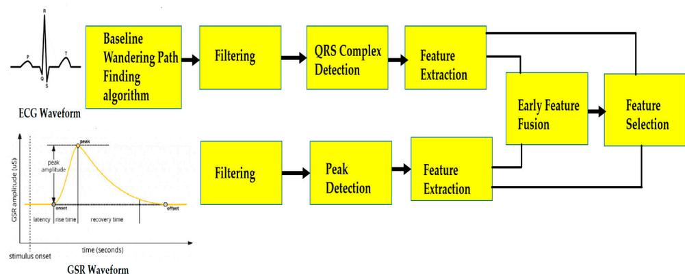
**Figure 2.** Block diagram for the preprocessing and feature fusion of ECG and GSR signals.
