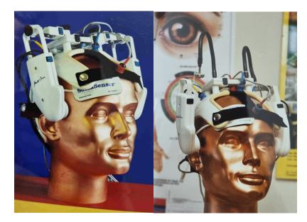
Figure 2. Multiparametric helmet construction in acupuncture research from 1997 (© Gerhard Litscher).
