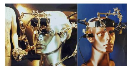
**Figure 3.** Simultaneous ultrasonic blood flow measurements in different cerebral arteries using a helmet construction developed in Graz in 2001 (© Gerhard Litscher).
