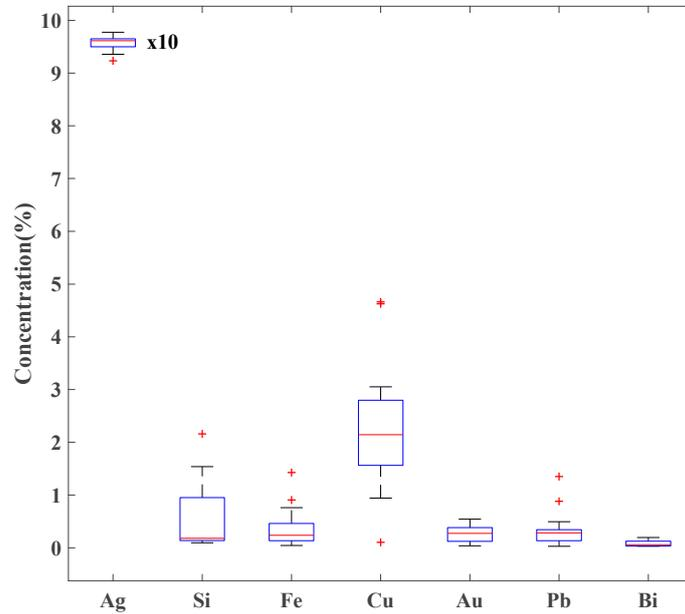
**Figure 2.** Box plot of the concentration values of the elements detected by the XRF. Silver values have been rescaled by a factor of 10.
