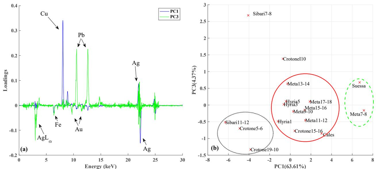
**Figure 6.** Loadings as a function of energies (keV) to determine which fluorescence peaks contribute most to the PCs. PC1 and PC3 give 68% cumulative variance.
