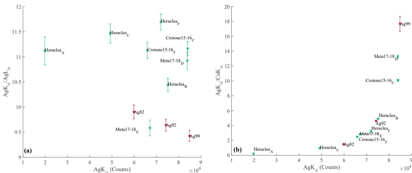
**Figure 4.** (a) Comparison of the ratio of silver  $\text{K}\alpha/\text{L}\alpha$  characteristic lines to the net area of Ag  $\text{K}\alpha$ ; (b) Comparison of the cross-ratio of silver  $\text{K}\alpha$  characteristic line to copper  $\text{K}\alpha$  vs. net area of Ag  $\text{K}\alpha$ .
