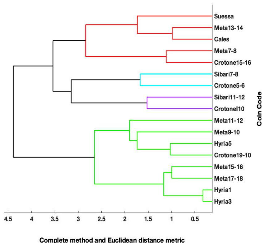
**Figure 8.** HCA on the XRF dataset using the complete linkage algorithm and the Euclidean metric.
