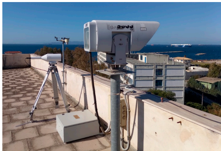
Figure 2. The MRV TS5000/155 FSO system, co-located with the BLS450 scintillometer and the ambient-weather WS-2000 weather station on the roof of the laboratory building of the Hellenic Naval Academy.
