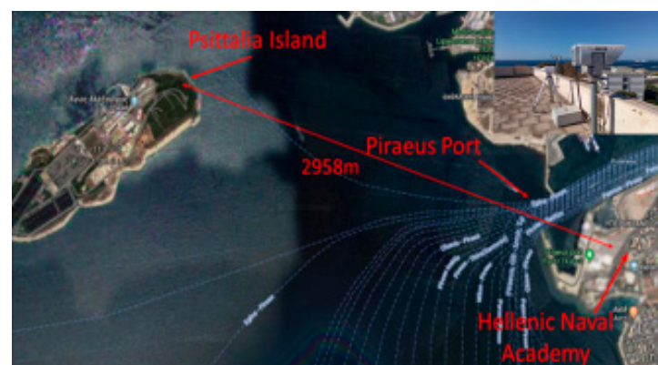
Figure 1. The laser-communications link located across the entrance to Piraeus port.
