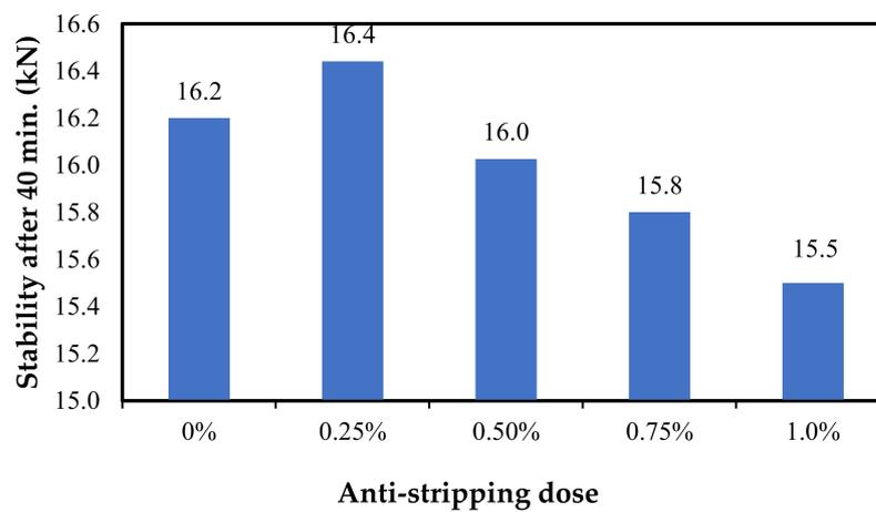
Figure 6. Marshall stability results after 40 min conditioning.
