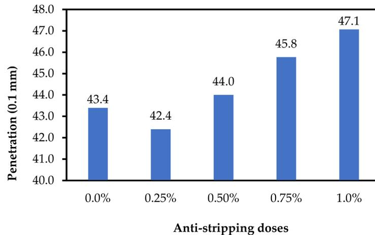
Figure 2. Penetration results of asphalt binders.
