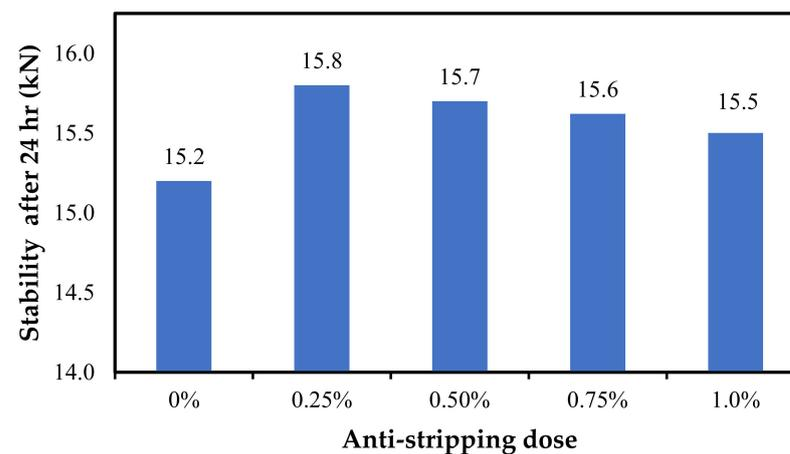
Figure 7. Marshall stability after 24 h conditioning.
