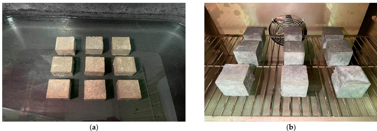
**Figure 4.** The process of saturation (a) and drying (b) of experimental samples.
