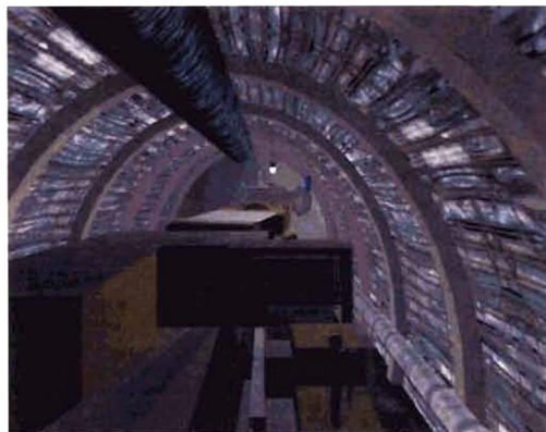
Figure 13. Image of virtual reality simulation model—AITEMIN roadheader simulation-operator's view [54].
