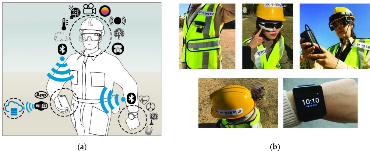
Figure 12. (a) Prototype of an interconnected sensor system associated with PPE [51]; (b) Embedded wearable systems tested at the mine site [52]. From top left to top right: sensor-equipped mine safety vest; miner wearing Recon Jet Smart Eyewear; miner using Epson Moverio BT-2200. From bottom left to bottom right: sensor-equipped safety helmet; smartwatch.
