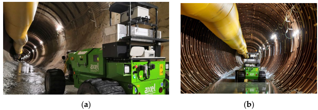
Figure 7. (a,b) The Axel Rover for inspections used in the “Maddalena niches” construction site.
