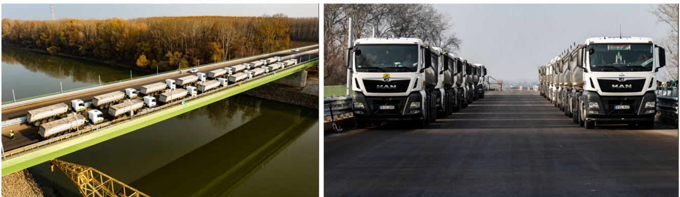
Figure 2. Bridge Truck loading test in 2 \times 2 configuration.
