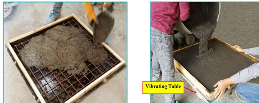
Figure 5. Pouring the mix into the plywood mold for slab specimens.
