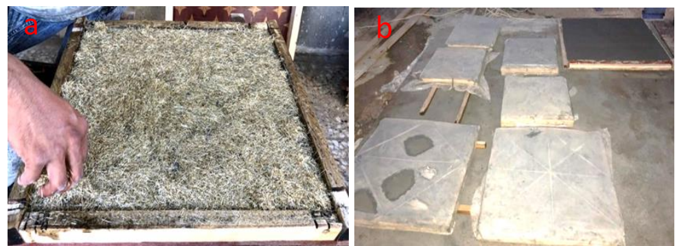
Figure 8. SIMCON laminates (a) fiber mats before coupling, (b) laminates after coupling to the slabs.
