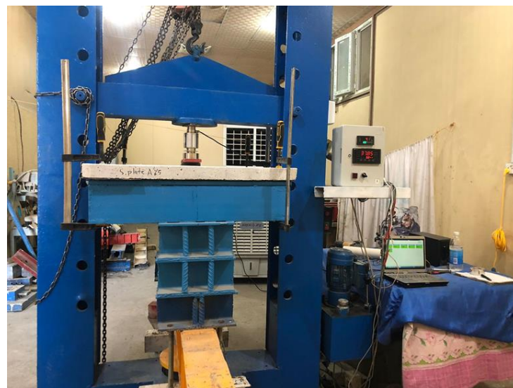
Figure 13. Set-up of the slab specimens.
