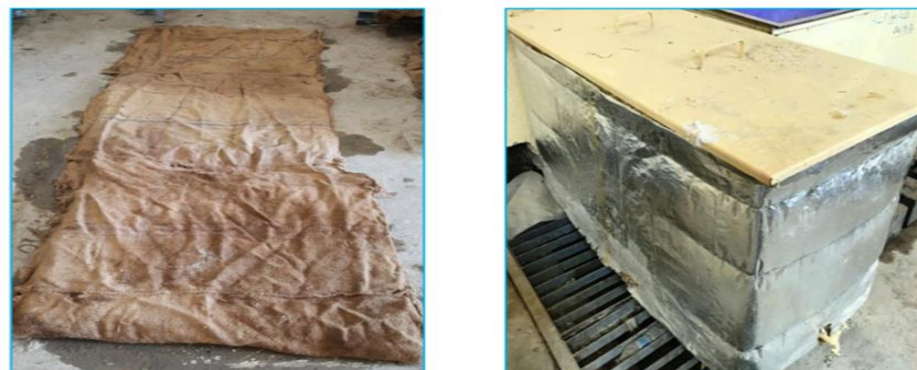
Figure 6. The curing process of slab specimens.
