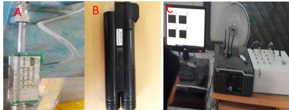
Figure 10. Instruments provided for testing, (A) LVDT of 50mm capacity, (B) Microscope for measuring the crack width, and (C) Data logger connecting to the computer to record data.
