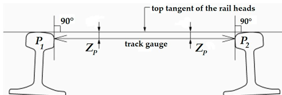
Figure 1. The measurement principle of the railway gauge parameter (drawn based on EN 13848-1 [14]).
