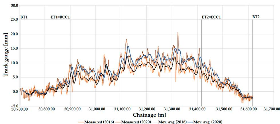
**Figure 20.** The longitudinal function of the track gauge on Line #1 (between Biatorbágy and Herceghalom railway stations), considering the measurement data in 2016 and 2020 and the sections with ECs. Moving average (mov. avg.) lines are added. The meanings of abbreviations are detailed in “Abbreviations” at the end of the paper.
