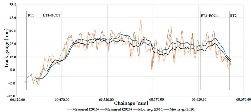
**Figure 21.** The longitudinal function of the track gauge on Line #11 (between Zirc and Eplény railway stations), considering the measurement data in 2016 and 2020 and the sections with ECs. Moving average lines are added. Moving average (mov. avg.) lines are added. The meanings of abbreviations are detailed in “Abbreviations” at the end of the paper.
