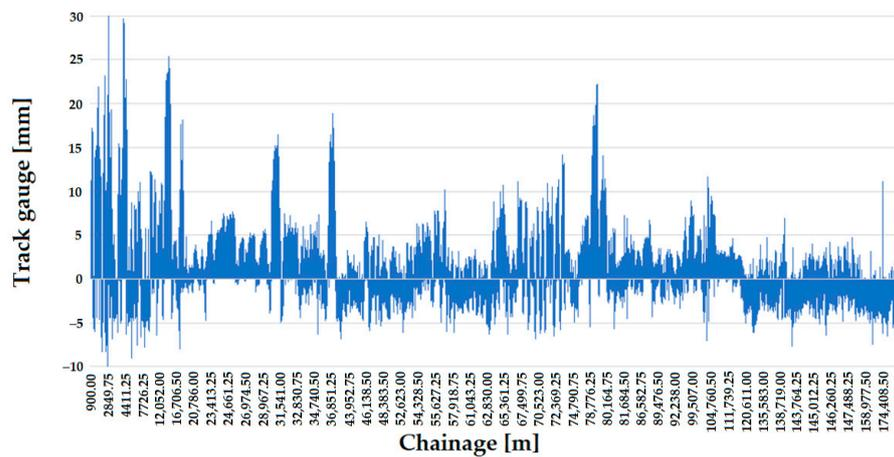
Figure 16. The longitudinal function of the track gauge on Line #1, considering the measurement data in 2011 and the sections with ECs.
