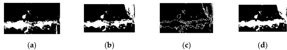
Figure 11. (a) Binary image before preprocessing; (b) binary image after preprocessing; (c) dilated edges with a line-shaped structural element; (d) connected area.
