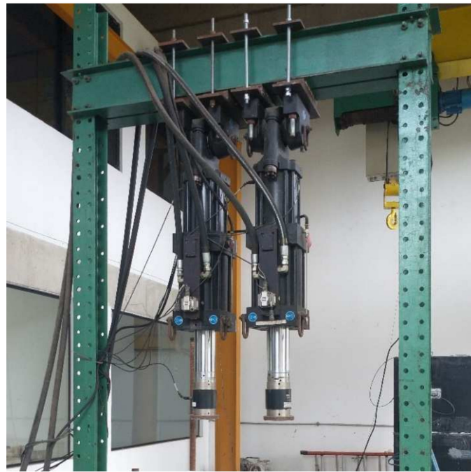
Figure 9. Hydraulic press for applying the load.
