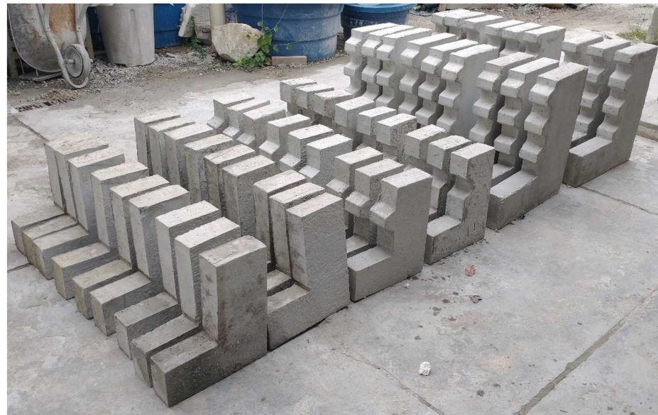
Figure 8. Dry joint specimens with recycled coarse aggregates concrete.
