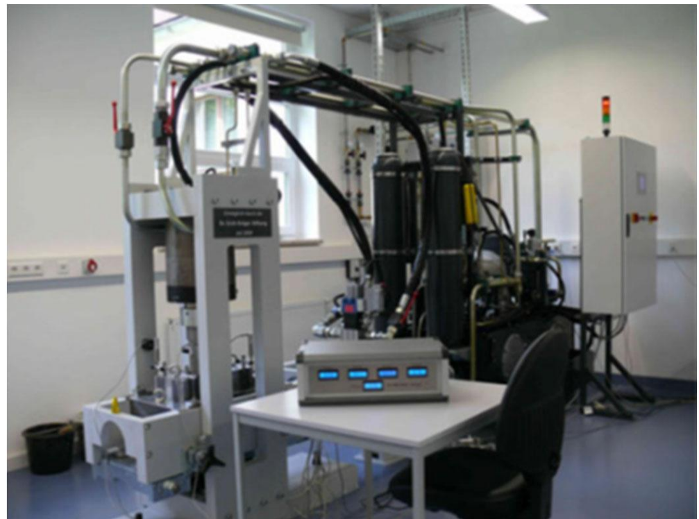
Figure 6. Astra test device: shear box device gs-1000.
