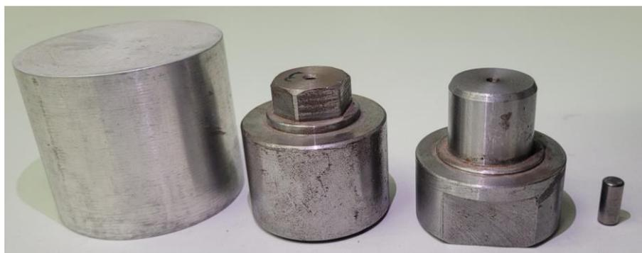
**Figure 7.** Weights applied for the print-free test.
