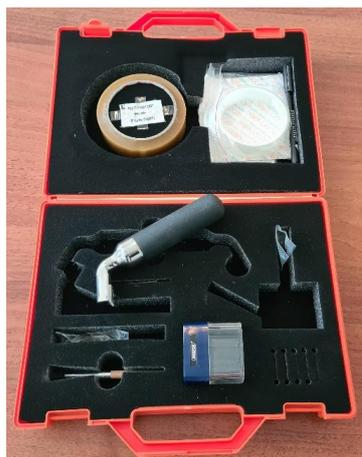
**Figure 8.** Elcometer 107 Cross-hatch cutter.
