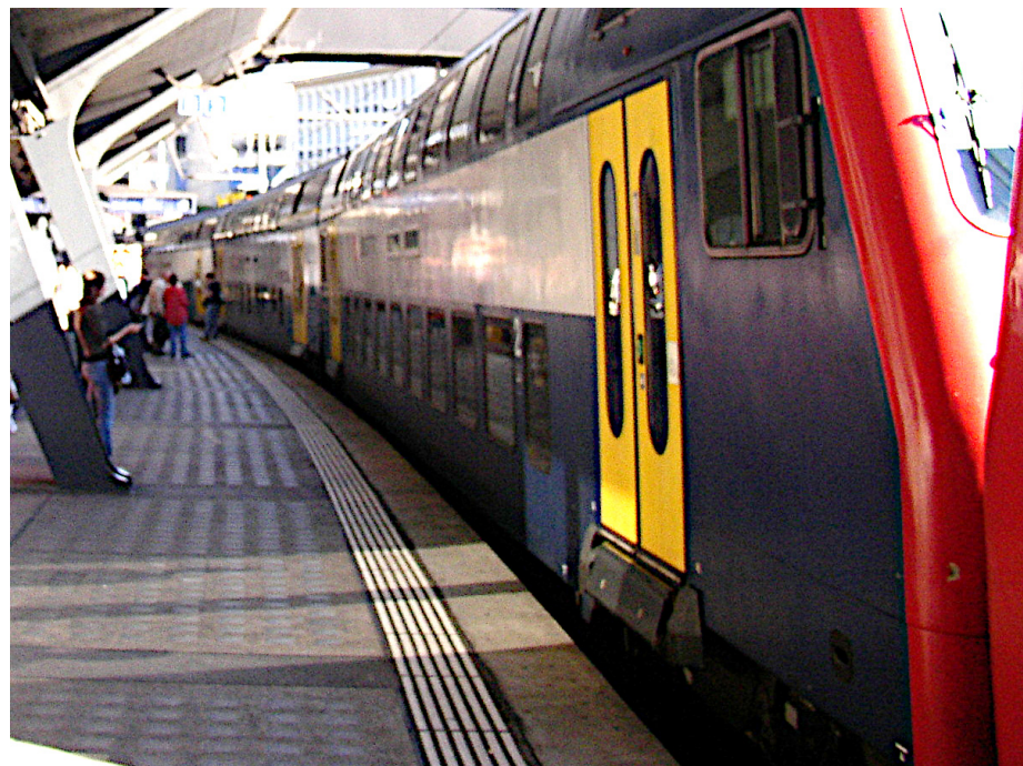
Figure 4. Train of S6 line (DPZ + Re450 in double traction) with fold-out steps opening to a horizontal position, about 200 mm wide, in Stadelhofen station (2006).
