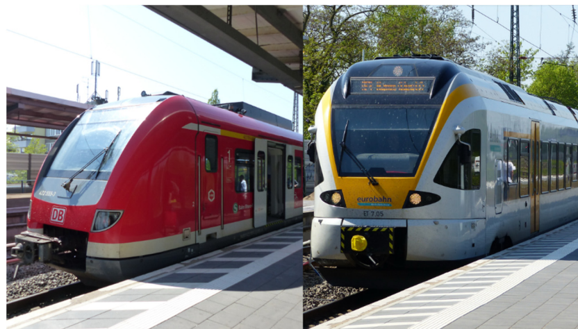
Figure 2. Trains BR 422 and Stadler Flirt at the newly modernized platform (April 2019), which is 760 mm high, at Castrop—Rauxel Hbf Station; different fits of entrance height are visible.
