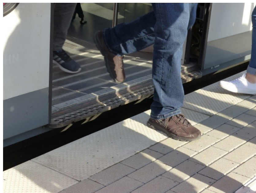
Figure 3. Door area of a double-decker car of Dresden CR at the platform, which is 550 mm high, at the Dresden Bischofsplatz stop.
