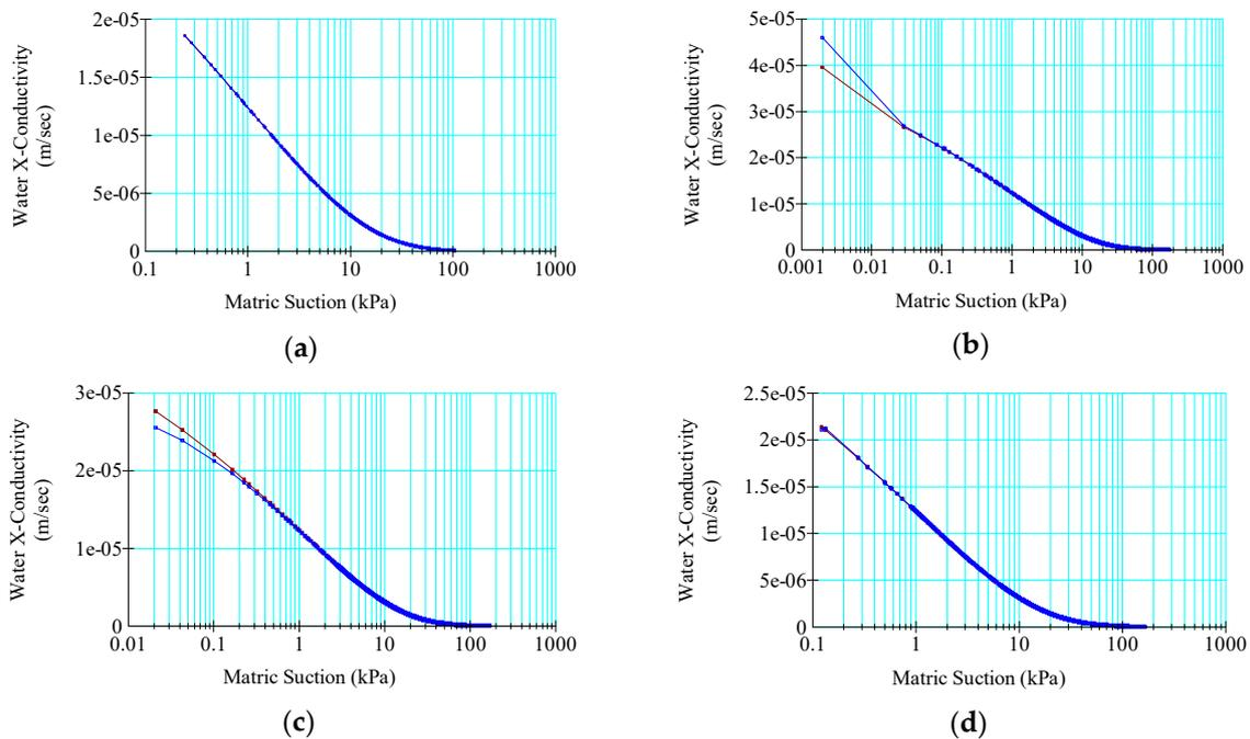
**Figure 3.** Water conductivity and matric suction without a drain under (a) steady-state, (b) instantaneous, (c) 10-day, and (d) 1 m per day drawdown.
