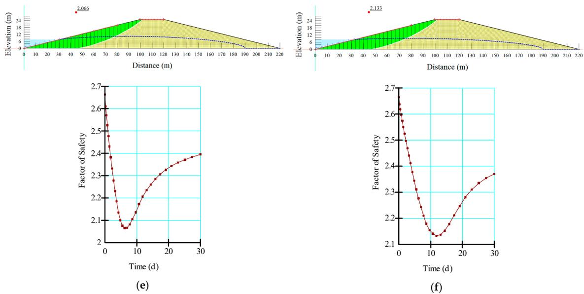
**Figure 5.** Trends in the factor of safety values for (a) 1:1 (V:H) without toe drain and instantaneous drawdown (b) 1:1 (V:H) without toe drain and 10-day drawdown (c) 1:1 (V:H) without toe drain and 1 m per day drawdown (d) 1:4 (V:H) with 30 m toe drain and instantaneous drawdown (e) 1:4 (V:H) with 30 m toe drain and 10-day drawdown (f) 1:4 (V:H) with 30 m toe drain and 1 m per day drawdown.
