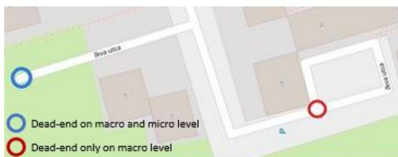
**Figure 3.** Node marked with a red circle is a dead-end on macro level and a three-way intersection on micro level.
