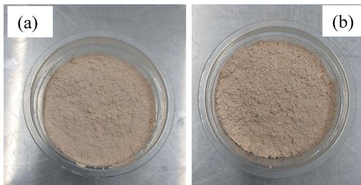
**Figure 3.** Calcinated clay after grinding (a) 800 °C/1 H/SL/60 (b) 800 °C/1 H/Su/60.
