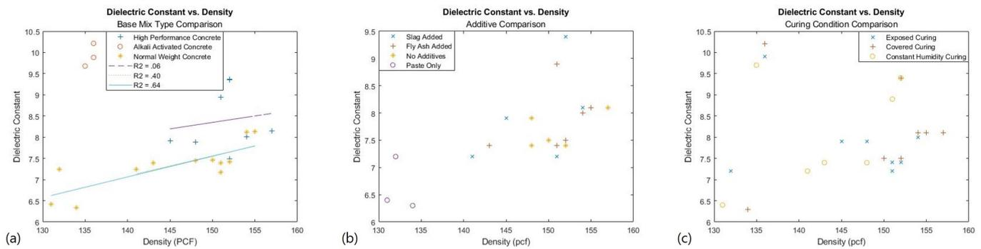
**Figure 8.** Dielectric constant vs. density (pounds per cubic foot, pcf) with breakdowns of base mix (a), additives (b), and curing condition (c).
