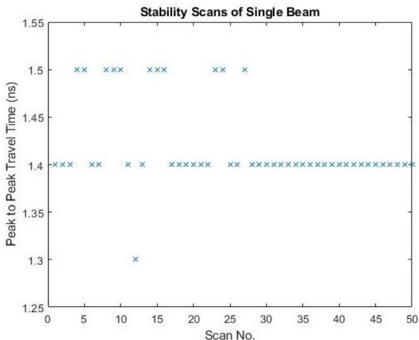
**Figure 5.** Plot of travel times to rebar in 50 scans of a single concrete beam. Note the resolution of 0.1 ns in the values.
