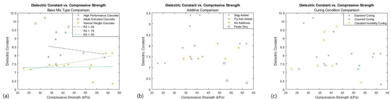
**Figure 7.** Dielectric constant vs. compressive strength (kPa) with breakdowns of base mix (a), additives (b), and curing condition (c).
