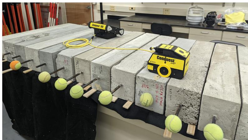
Figure 2. Single-line scanning setup showing adjacent beam placement.
