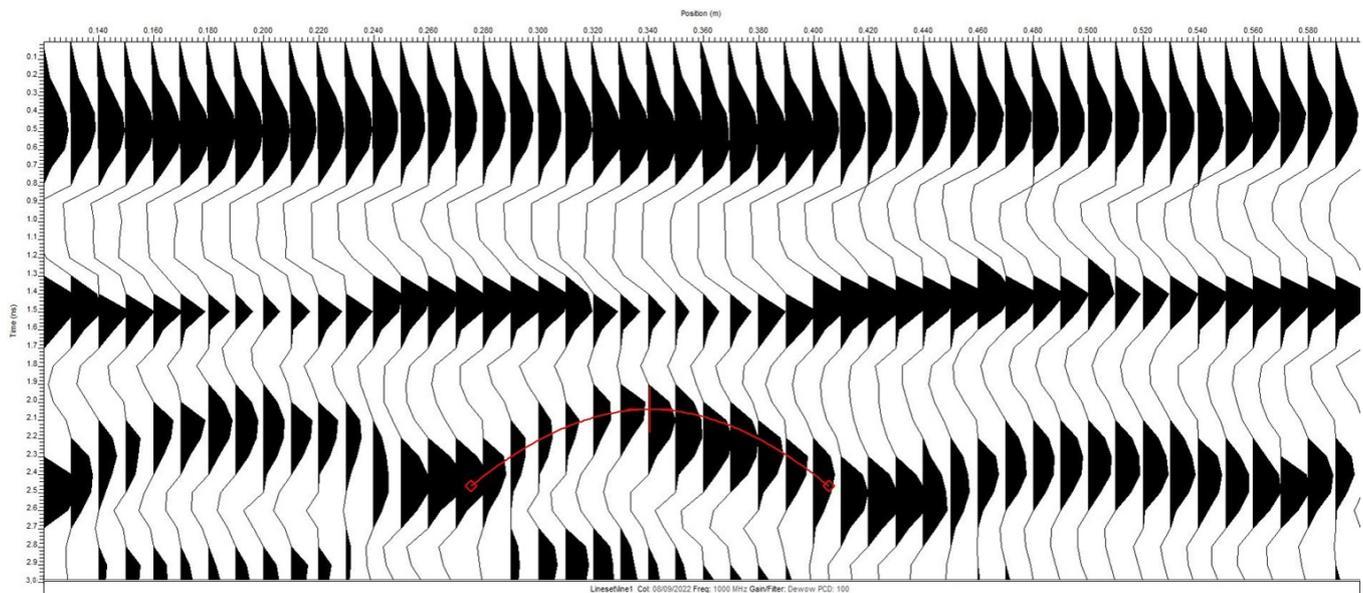
**Figure 4.** Radargram of continuous scan in EKKO V6, with one hyperbola shown. Note the different hyperbolas from the rebar in each beam.
