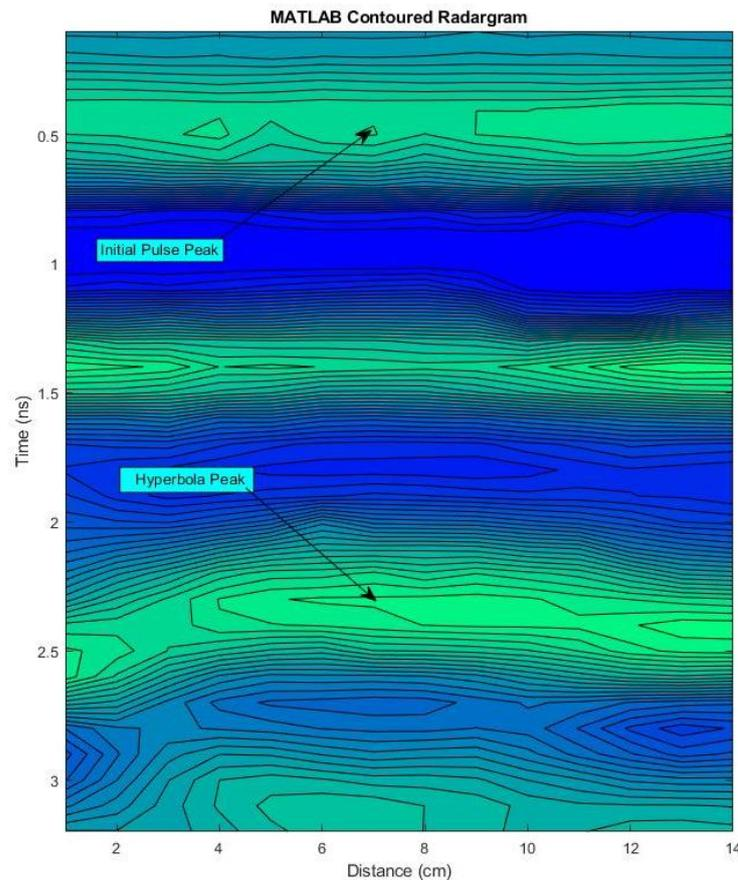
**Figure 3.** Radargram of single beam section shown in MATLAB using a contour plot. Note peak of hyperbola around 7 cm and 2.25 ns depth.
