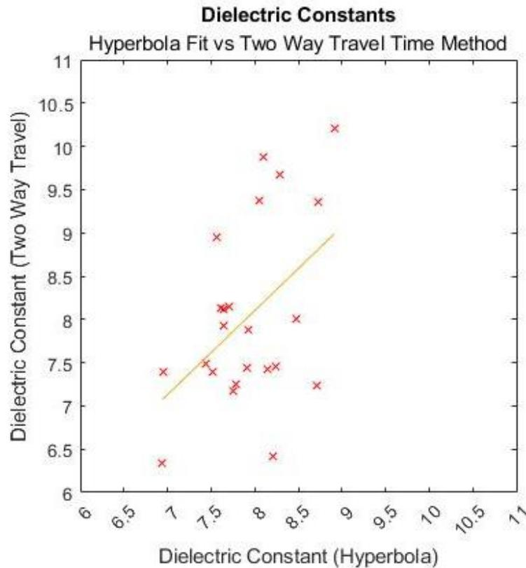
**Figure 6.** Correlation plot of dielectric constants found with hyperbola fitting and two-way travel time.
