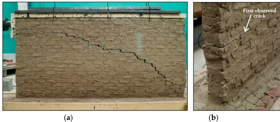
Figure 9. Wall 2: (a) near failure; (b) first crack at the transition between wet and dry regions.
