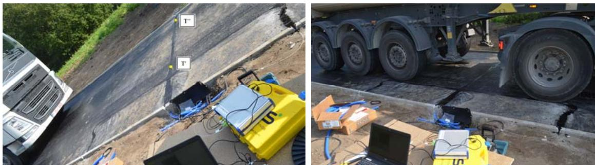
**Figure 8.** Monitoring of FBGs during the second day during the construction of the second base layer of the CyPaTs bicycle path.
