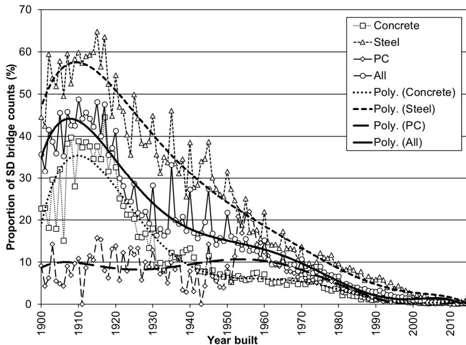
Figure 6. Distribution of the proportion of structurally deficient bridges.
