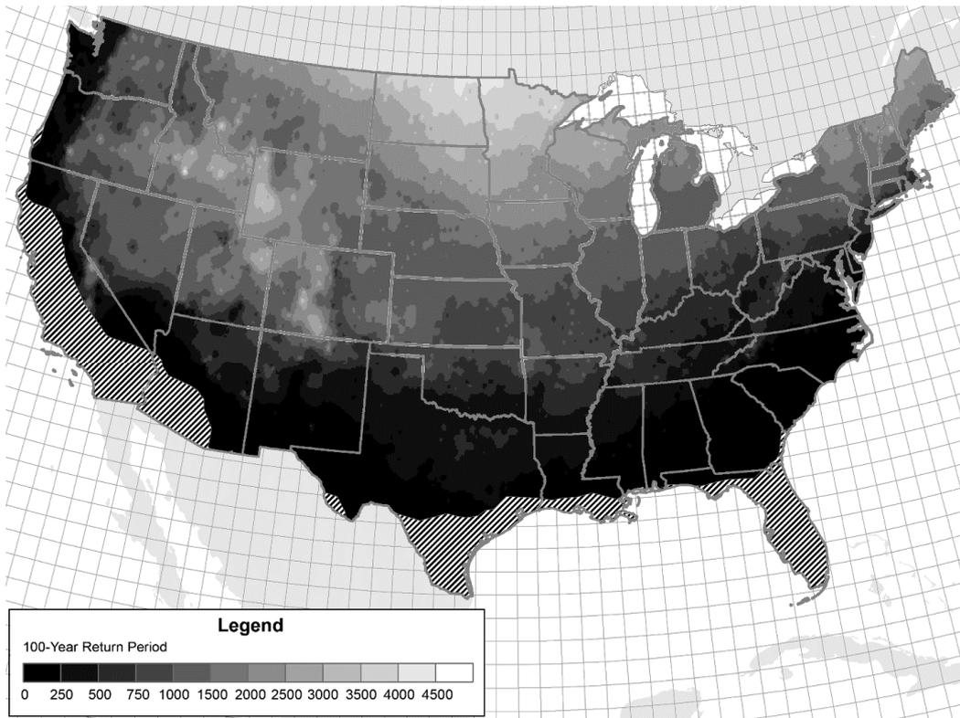
Figure 8. Freezing severity of winter and frost depth [20]. (Excerpt reprinted with permission).
