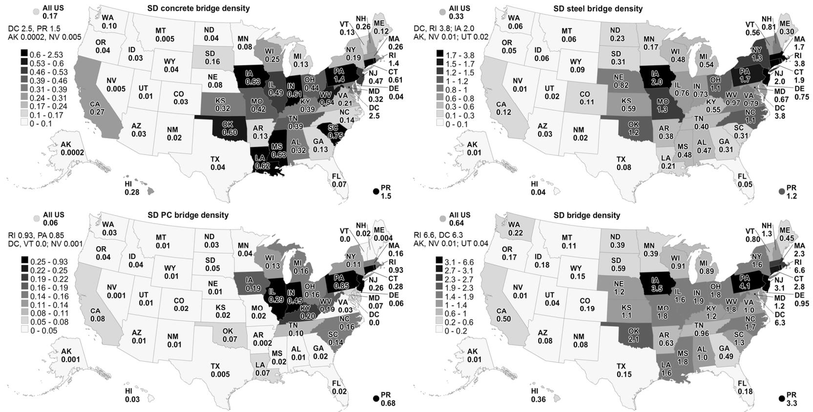
Figure 4. Density (count/10<sup>8</sup> m<sup>2</sup>) of structurally deficient bridges by state.
