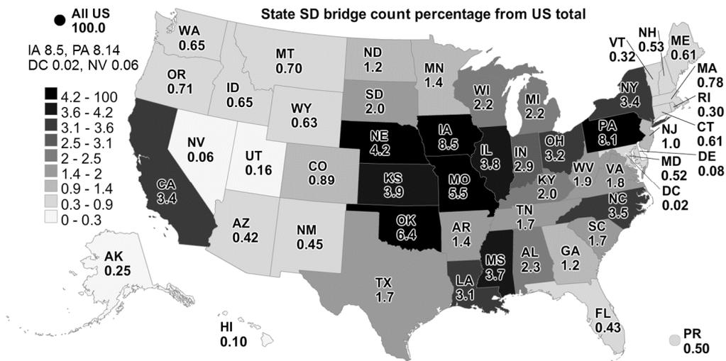
Figure 2. Percentage distribution of state structurally deficient bridge counts from U.S. total.
