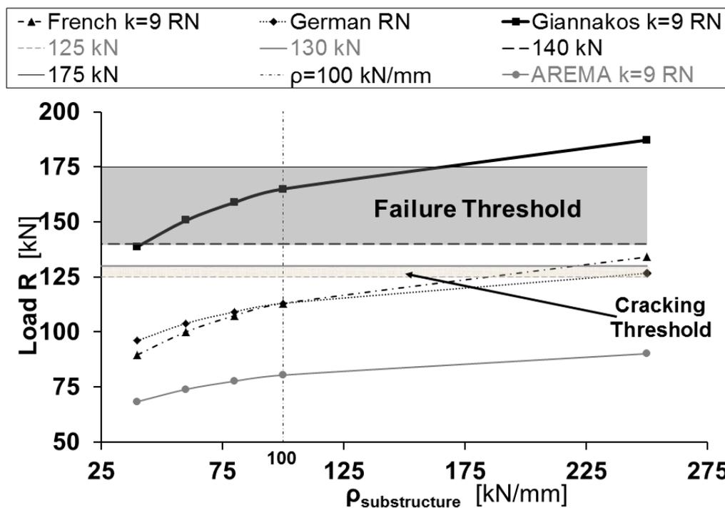
**Figure 1.** The results of the four methods (American, German, French, and Giannakos) for the loading and the strength of the U3/U2 concrete sleeper with RN fastenings, after a sensitivity analysis for the fluctuation of  $q_{subgrade}$  [15].
