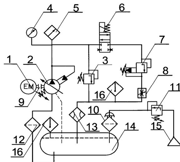
**Figure 4.** Scheme of the laboratory hydraulic system for testing CPAP. 1—electric motor; 2—pump CPAP; 3—safety valve; 4—manometer; 5—pressure transducer; 6—electromagnetic distributor; 7—pressure regulator of indirect action; 8—damper of variable resistance; 9—elastic coupling; 10—intake filter; 11—air pressure regulator; 12—intake filter; 13—flow converter; 14—pressure tank; 15—pressure air source; 16—temperature converter.
