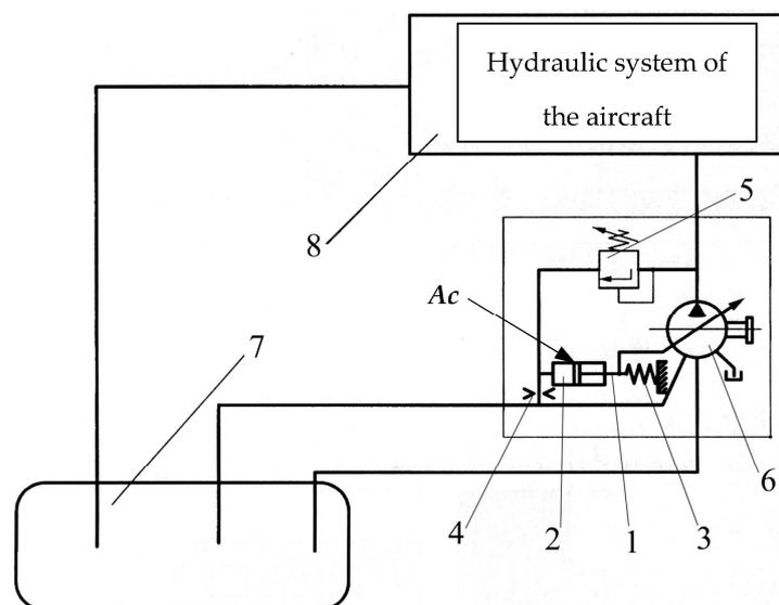
**Figure 2.** Functional diagram of a constant pressure pump. 1—piston rod; 2—cylinder; 3—spring; 4—muffer; 5—distributor for regulation; 6—hydraulic pump; 7—pressure tank; 8—actuators of working fluid.
