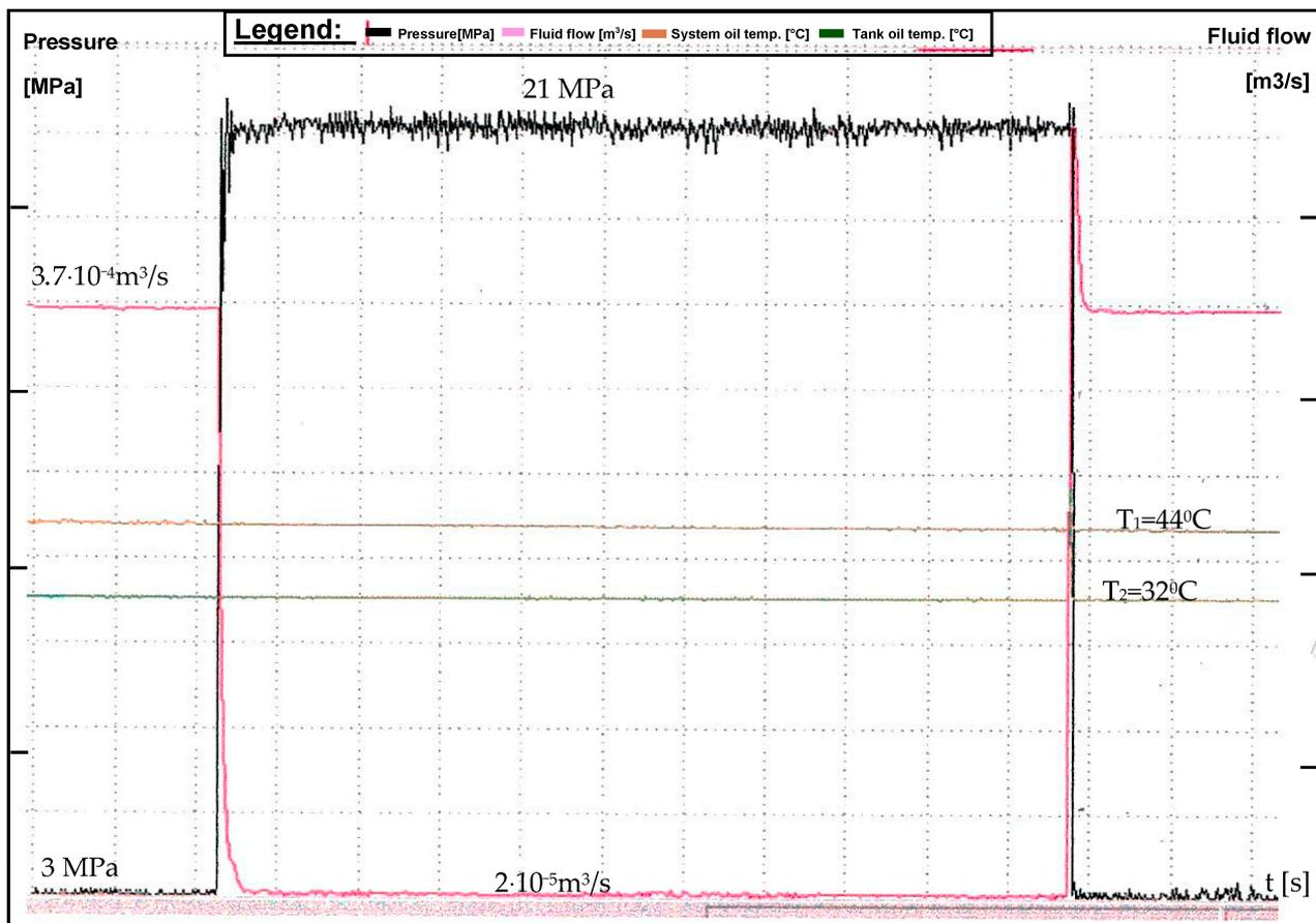
**Figure 5.** Diagram of the change in flow when the pressure changes from  $p_r = 3$  MPa to  $p_{max} = 21$  MPa (pressure range from 3 to 23 MPa, the cut-off value is 2 MPa).
