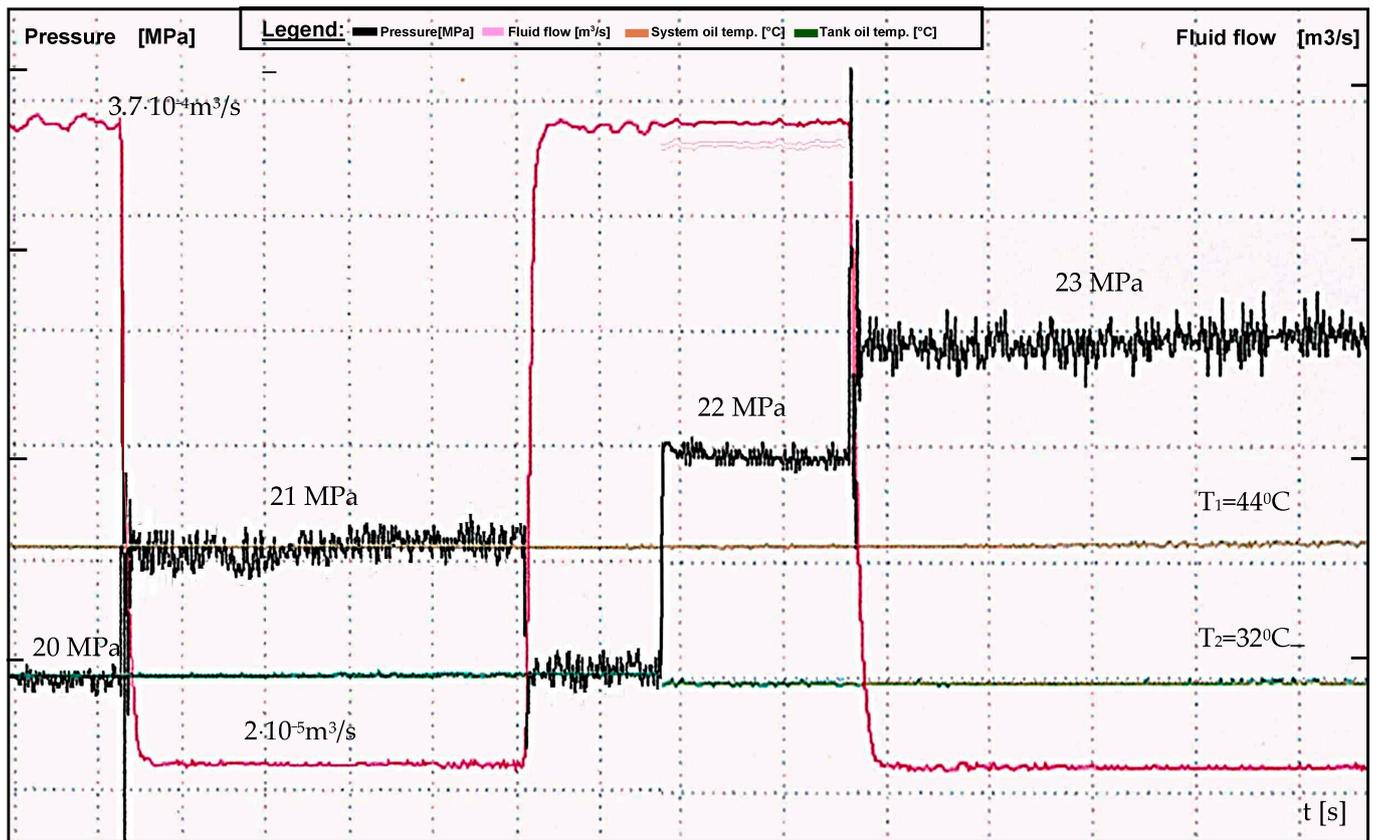
**Figure 7.** Diagram of the change in flow when the pressure changes in two levels, from 20 MPa to 21 MPa and from 22 MPa to 23 MPa (the pressure range is from 13 to 23 MPa; the value of the division on the diagram is 1 MPa).
