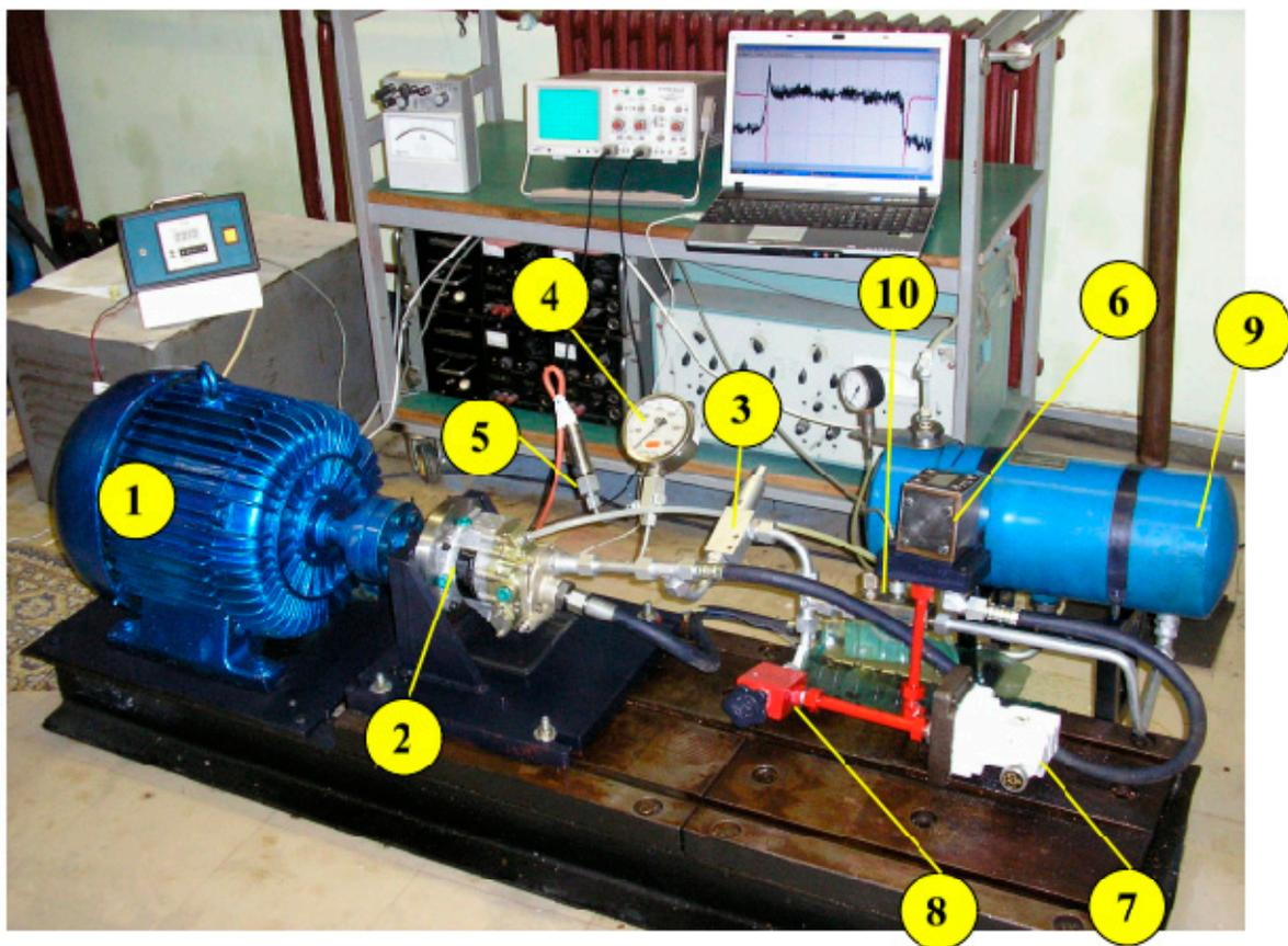
**Figure 3.** The laboratory hydraulic system for testing CPAP. 1—electric motor; 2—hydraulic pump; 3—safety valve; 4—manometer; 5—pressure transducer; 6—electromagnetic distributor; 7—pressure regulator; 8—muffler; 9—flow converter; 10—pressure tank.
