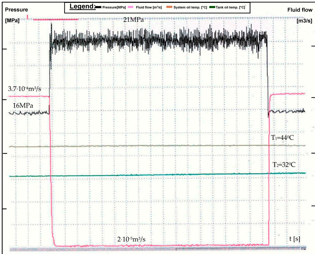
**Figure 6.** Diagram of the flow rate change when the pressure changes from  $p_r = 16$  MPa to  $p_{max} = 21$  MPa (pressure range 6 to 23 MPa; the value of the partition is 1.7 MPa).
