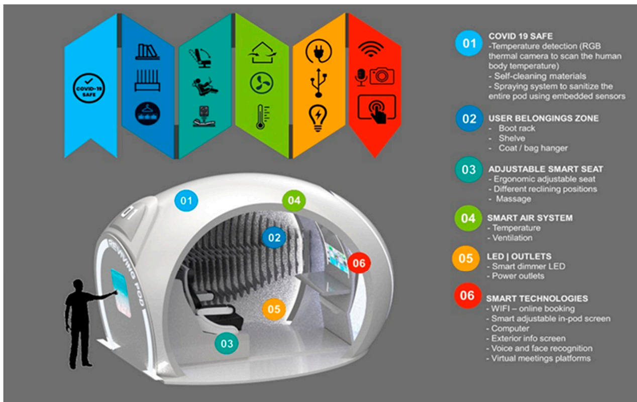
Figure 12. Diagram indicating COVID-19 precautions in the pod’s design, illustrating the personal belongings zone, adjustable smart seat, LED outlets, and various smart technologies used within the Reviving Pod, as designed by the authors.
