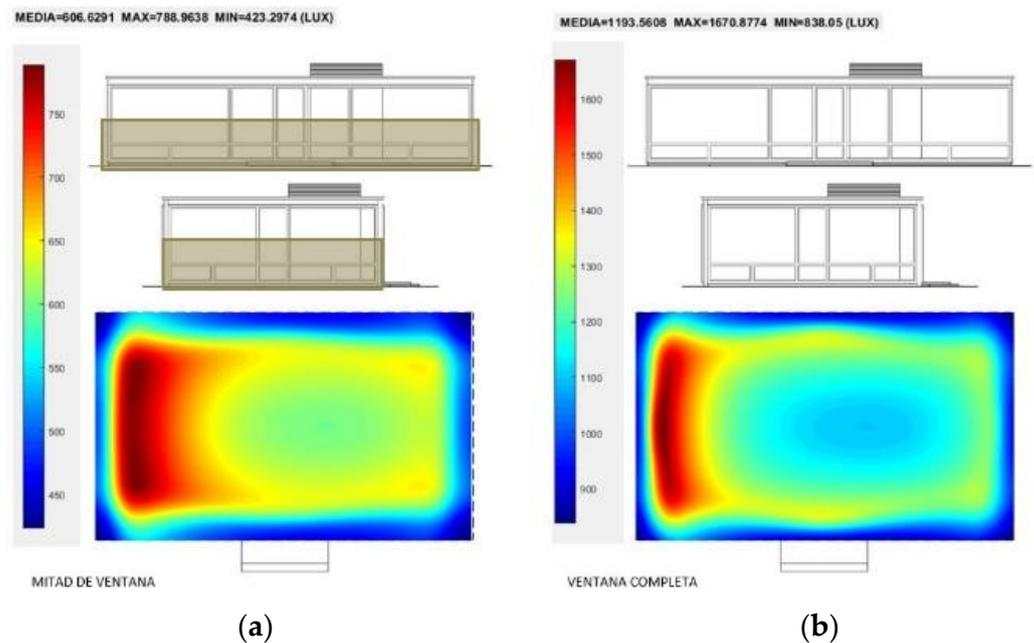
**Figure 14.** Glass House results in plan. (a) Half height windowsill at 1.8 m. (b) Full window.
