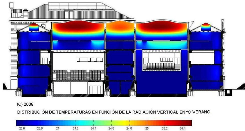
Figure 17. Vertical distribution of temperatures in deg. C, during summer.
