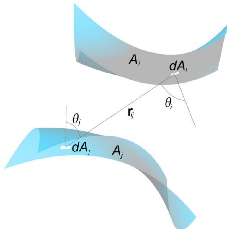
**Figure 1.** Arrangement of surface-source elements. Source: Salguero-Andujar.
