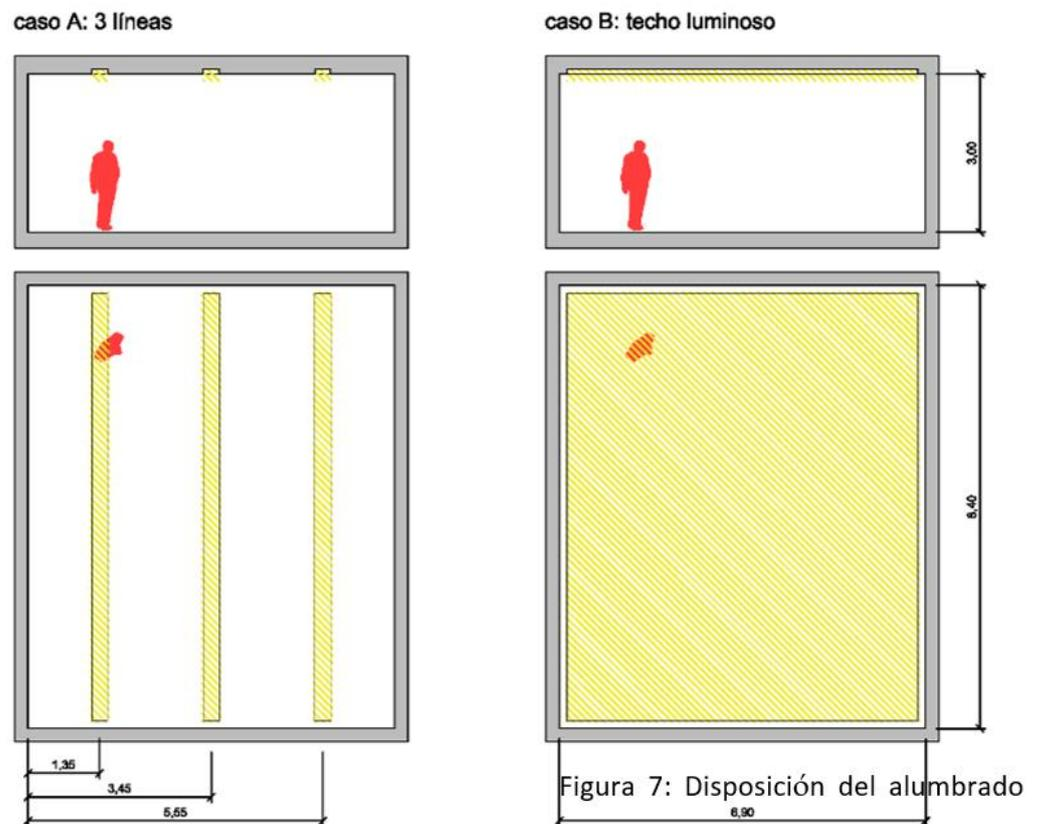
Figure 25. Linear lighting (right) versus surface lighting (left).
