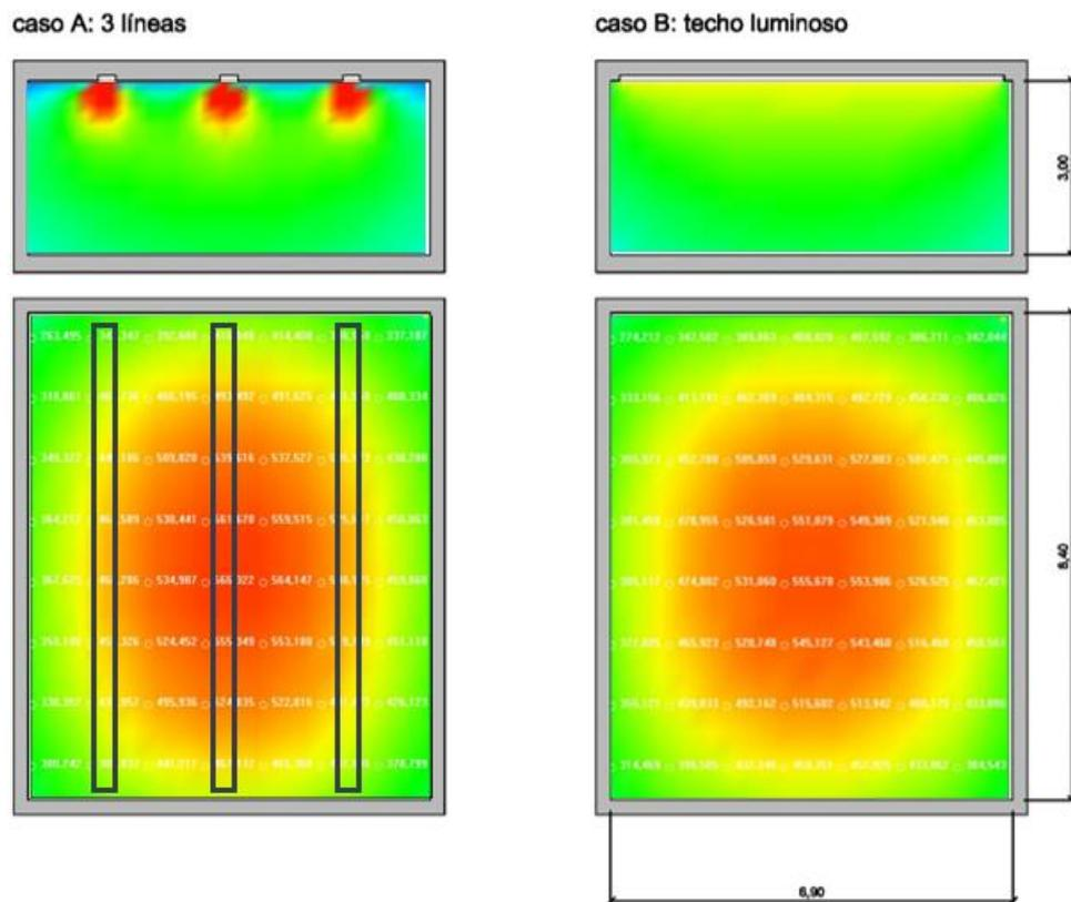
Figure 27. Surface lighting vs. linear by Lorenzo Muro.
