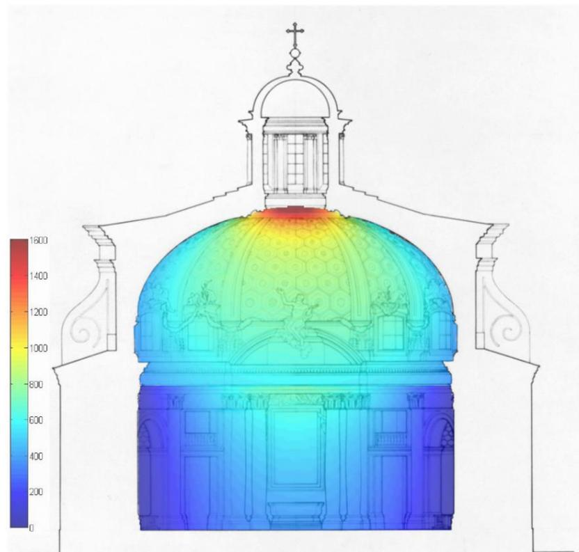
**Figure 10.** Daylight cross section of the church.
