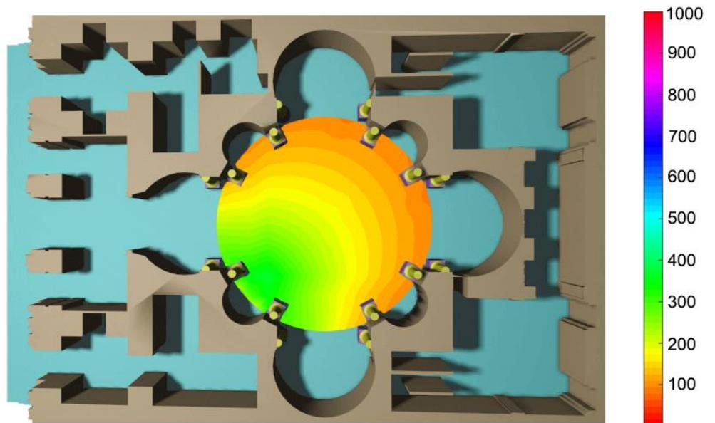
**Figure 4.** Simulations for the typical spring sunny day values in lux. This case occurs in 74% of the total time (76% during harvest). The distribution is reversed in the south–north axis at 8.45 h. Source: Authors.
