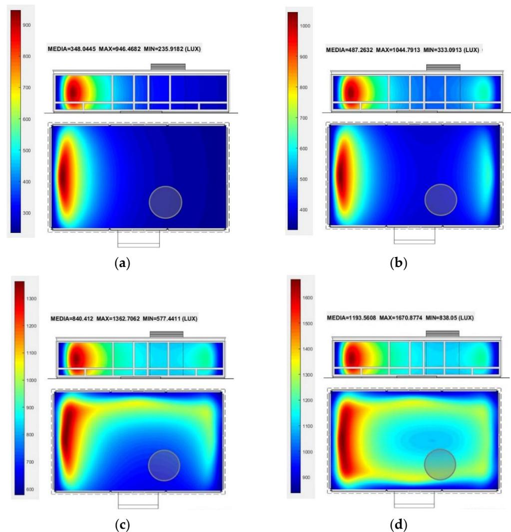
**Figure 13.** Lighting breakdown following the four façades of the building. (a) Glazing only on the left side. (b) Left and right sides. (c) Both sides and glazing on the upper side. (d) Glazing on the four sides.
