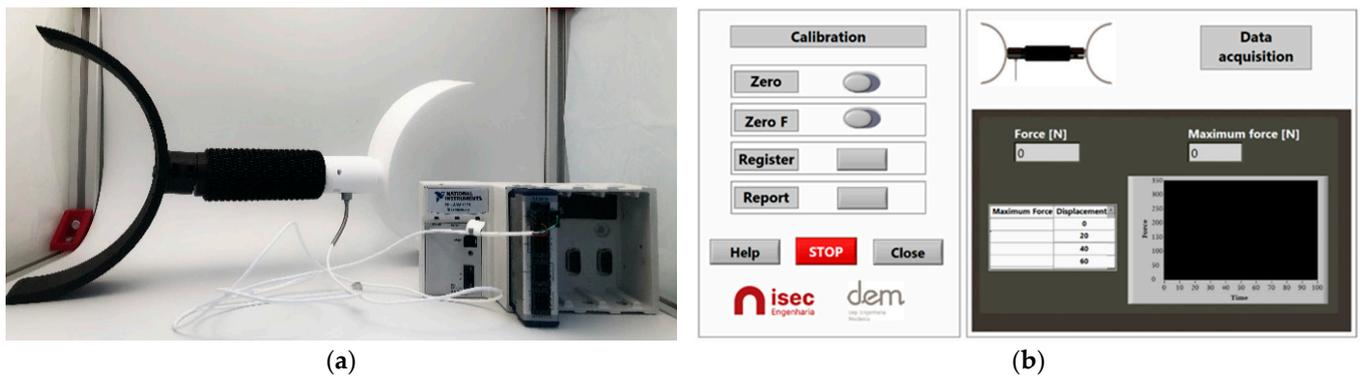
Figure 8. (a) Instrumented device; (b) Interface of Labview program to connect the load cell.
