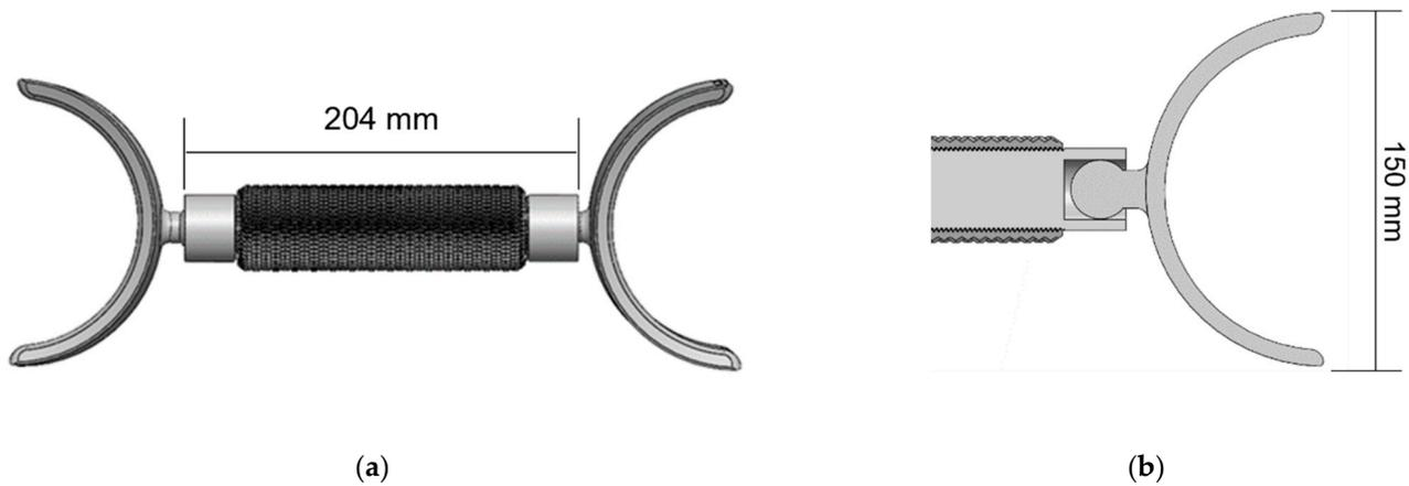
**Figure 2.** 3D model of the mechanical device: (a) Global visualization; (b) Detail of pivot system.
