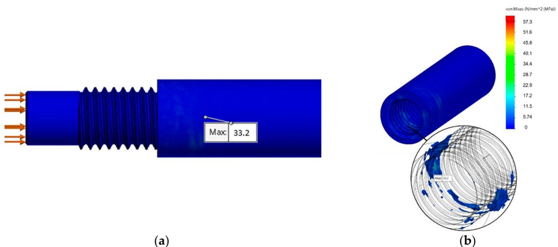
Figure 15. Distribution of von Mises stress for the instrumented device: (a) View of the global model; (b) Detail of von Mises stress distribution in the contact region.
