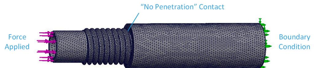
**Figure 11.** Visualization of the mesh, boundary conditions, and force applied in the finite element model of the instrumented device.
