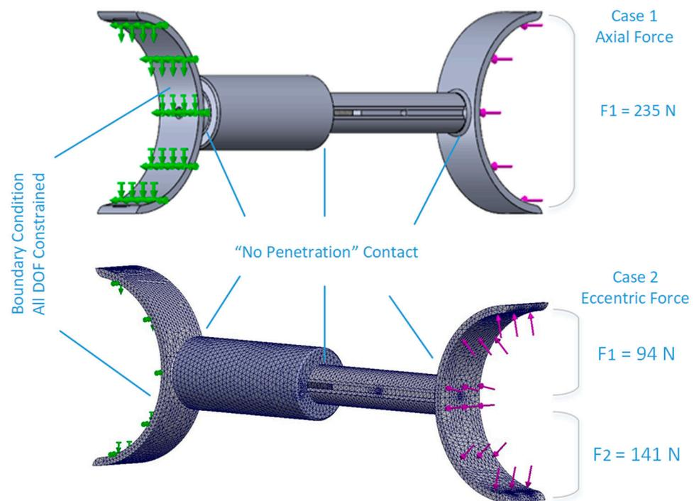
**Figure 12.** Load and boundary conditions for both situations.
