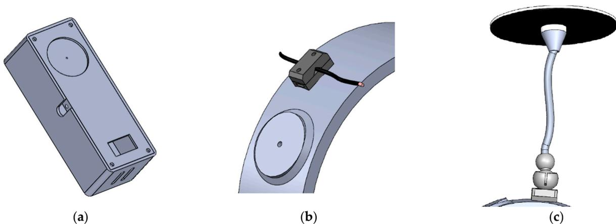
**Figure 5.** Add-ons: (a) Control unit; (b) Anchoring the camera; (c) Mirror anchor.
