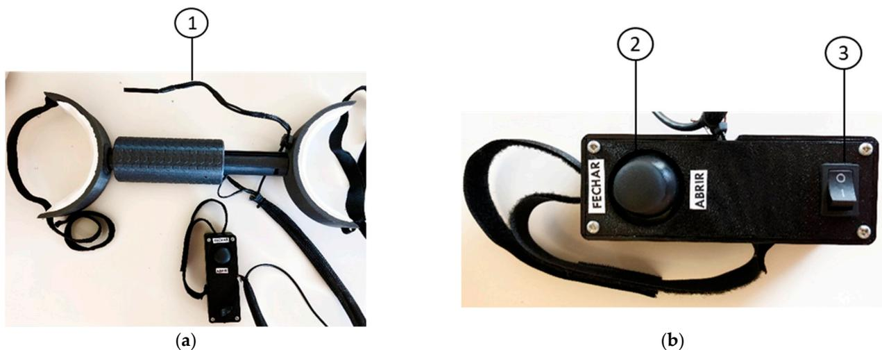
Figure 10. (a) Motorised device: (1) Camera with adjustable cable; (b) Detail of the command unit: (2) Button on/off; (3) Joystick.
