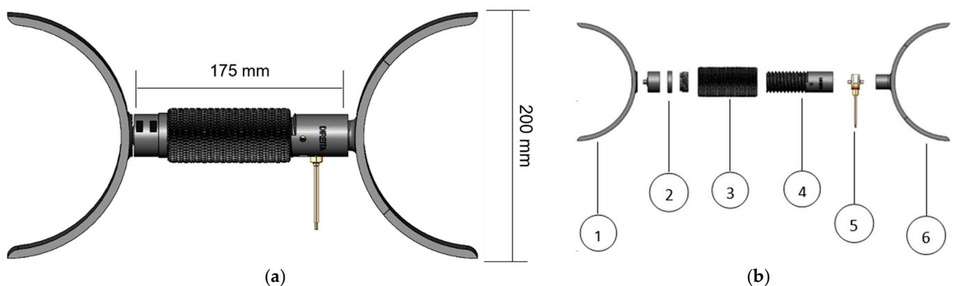
**Figure 3.** 3D model of the instrumented device for force measurement: (a) Global visualization; (b) Detail with components, (1)—fixed claw, (2)—fixed side element, (3)—central element, (4)—mobile side element, (5)—load cell, (6)—instrumented claw.
