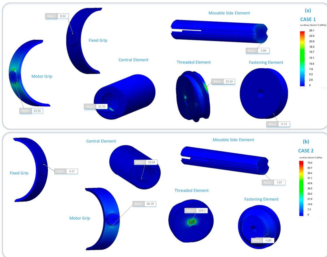
**Figure 16.** Distribution of von Mises stress in the mechanical components: (a) Load Case 1—axial force; (b) Load Case 2—eccentric force.
