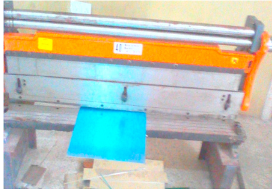
Figure S4: Folding marked out aluminum sheet by metal folding machine.
