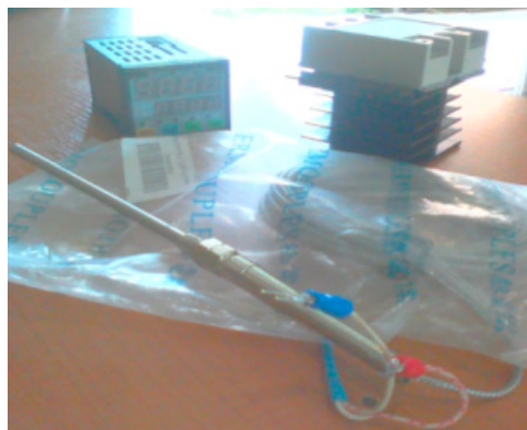
Figure S2: Temperature sensor, solid state relay and temperature controller.
