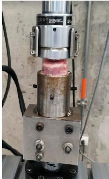
**Figure 2.** Compression test of porcine vertebrae.
