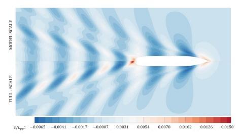
Figure 12. Comparison between model scale and full scale for wave elevation in calm water.
