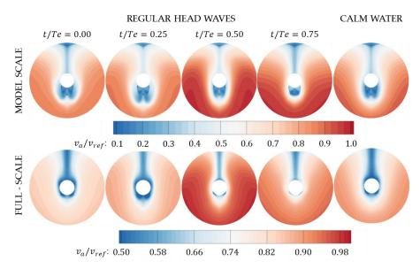
**Figure 15.** Comparison between model scale and full scale for axial velocity in the propeller in regular head waves for  $\lambda/L_{pp} = 1.951$  and  $H_w/L_{pp} = 0.032$ . Section at propeller plane.
