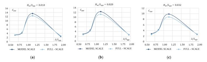
**Figure 9.** Comparison between model-scale and full-scale curves for wave added resistance coefficient in the case of (a)  $H_w/L_{pp} = 0.010$ , (b)  $H_w/L_{pp} = 0.020$ , and (c)  $H_w/L_{pp} = 0.032$ .
