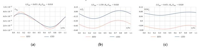
**Figure 5.** Comparison between CFD and EFD curves for (a) total resistance coefficient in wave amplitude, (b) heave amplitude, and (c) pitch amplitude for  $\lambda/L_{pp} = 0.651$  and  $H_w/L_{pp} = 0.010$ .
