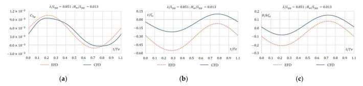
**Figure 6.** Comparison between CFD and EFD curves for (**a**) total resistance coefficient in wave amplitude, (**b**) heave amplitude, and (**c**) pitch amplitude for  $\lambda/L_{pp} = 0.851$  and  $H_w/L_{pp} = 0.013$ .
