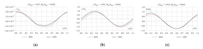
**Figure 8.** Comparison between CFD and EFD curves for (a) total resistance coefficient in wave amplitude, (b) heave amplitude, and (c) pitch amplitude for  $\lambda/L_{pp} = 1.951$  and  $H_w/L_{pp} = 0.032$ .
