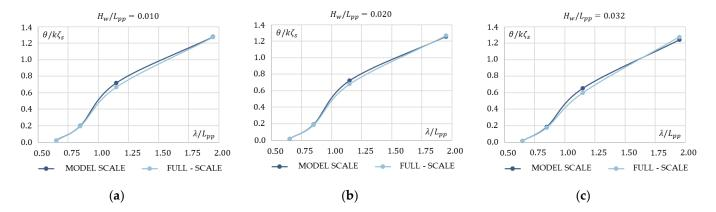
**Figure 11.** Comparison between model-scale and full-scale curves for pitch amplitude in the case of (a) $H_w/L_{pp} = 0.010$ , (b)  $H_w/L_{pp} = 0.020$ , and (c)  $H_w/L_{pp} = 0.032$ .
