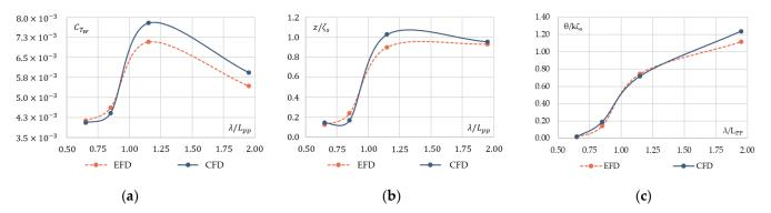
**Figure 4.** Comparison between CFD and EFD curves for (a) total resistance coefficient in waves, (b) heave amplitude, and (c) pitch amplitude.
