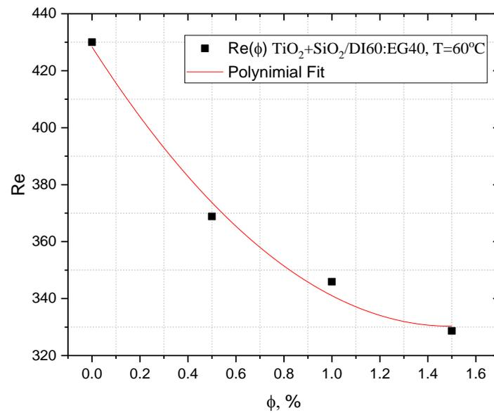
Figure 3. Reynolds number versus  $\text{TiO}_2\text{:SiO}_2\text{/EG/DI}$  nanofluid volumetric concentration.
