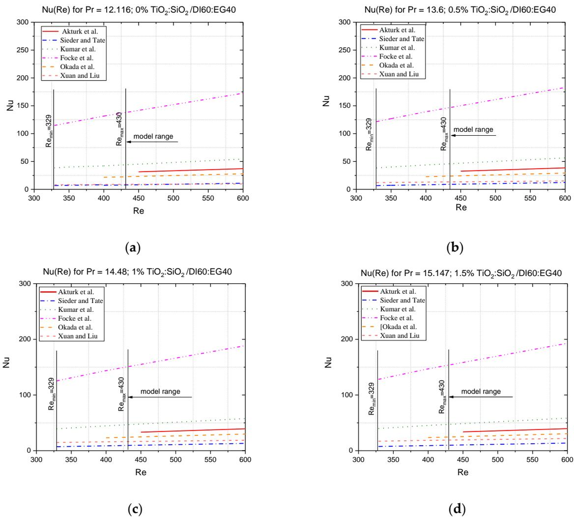
Figure 4. Variation in the Nusselt number of  $\text{TiO}_2\text{:SiO}_2\text{/DI:EG}$  hybrid nanofluid during flow through the PHE system versus Reynolds number for the following vol. concentrations: (a) 0%; (b) 0.5%; (c) 1.0%; (d) 1.5% [27–31,39].
