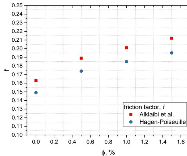
Figure 7. Friction factor versus  $\text{TiO}_2\text{:SiO}_2/\text{EG:DI}$  nanofluid concentration [4].
