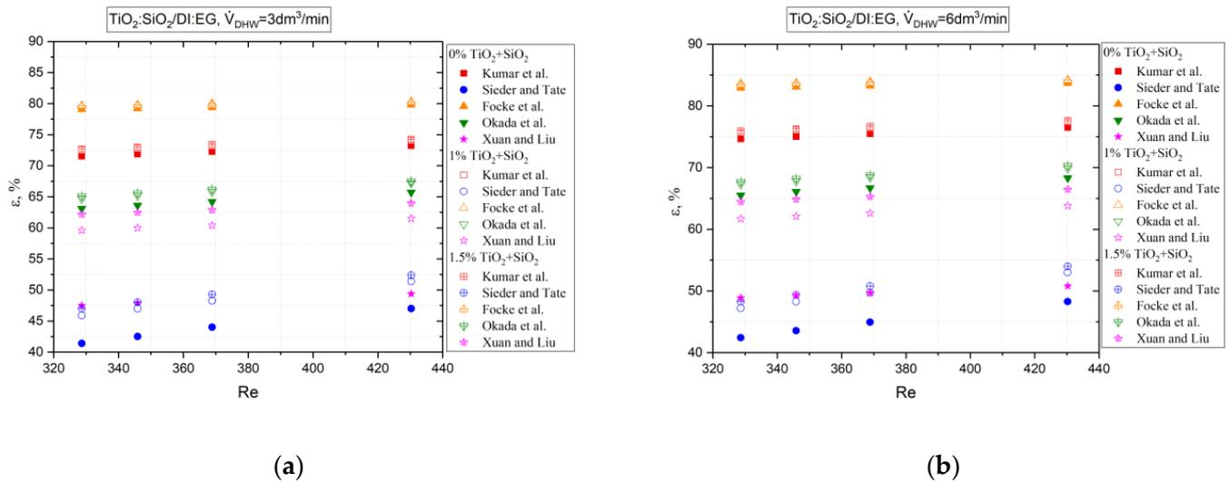
**Figure 6.** Effectiveness of PHE for  $\text{TiO}_2 + \text{SiO}_2/\text{DI:EG}$  hybrid nanofluid versus Reynolds number for varying Nusselt models and volumetric flow of (a)  $\dot{V}_{nf} = 3 \text{ dm}^3/\text{min}$  and (b)  $\dot{V}_{nf} = 6 \text{ dm}^3/\text{min}$  [28–31,39].
