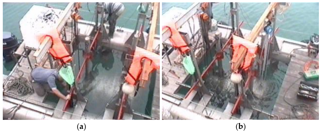
Figure 7. The duct scale models D3 (a) and D4 (b) fixation at the lower level with the highest part about 0.5 m below the water surface.
