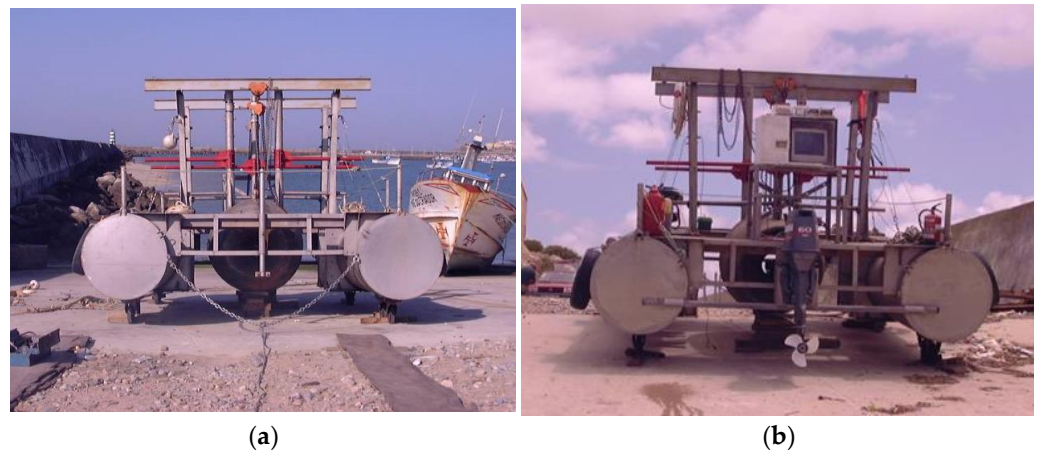
Figure 3. Front (a) and backward (b) views of the raft with the duct scale model D3 at a higher level at the naval dockyard ramp.
