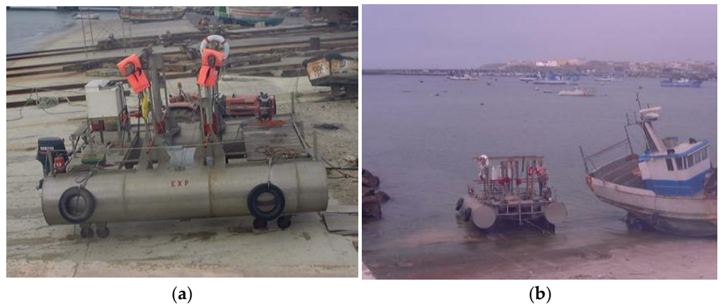
Figure 4. (a) Lateral view of the platform with the raft and the duct scale model D2 at the naval dockyard ramp and (b) image of the platform entering water or arriving at the dockyard ramp.
