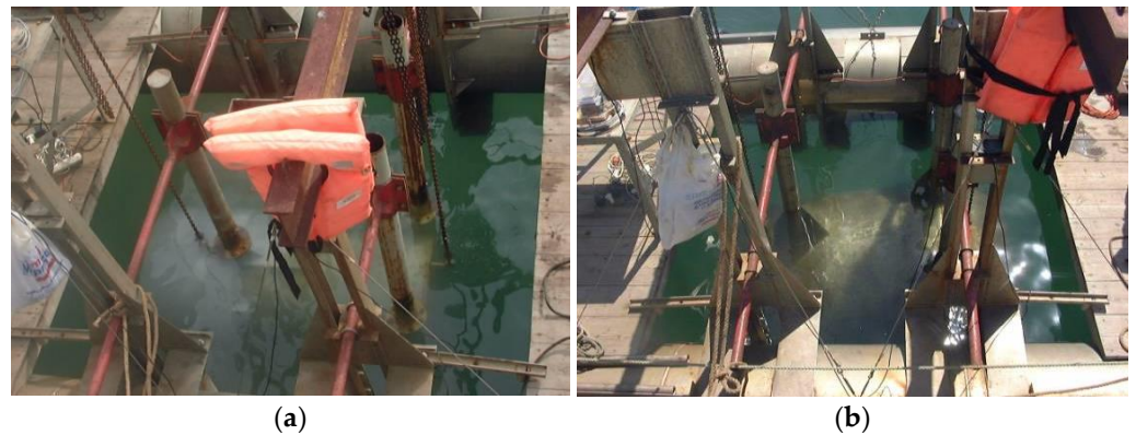
Figure 6. The duct scale models D2 (a) and D4 (b) at the lower level (totally immersed in the water) with the highest part about 0.5 m below the water surface, when the platform was tied to the quayside.
