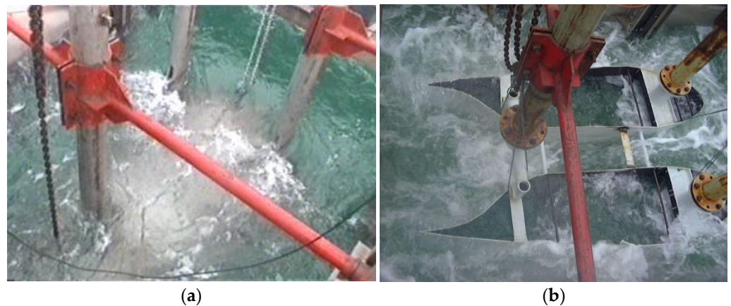
Figure 9. Duct scale model D3 dragged immersed by the raft in motion (a); the scaled planar profile of duct model D3 dragged immersed by the raft in motion (b).
