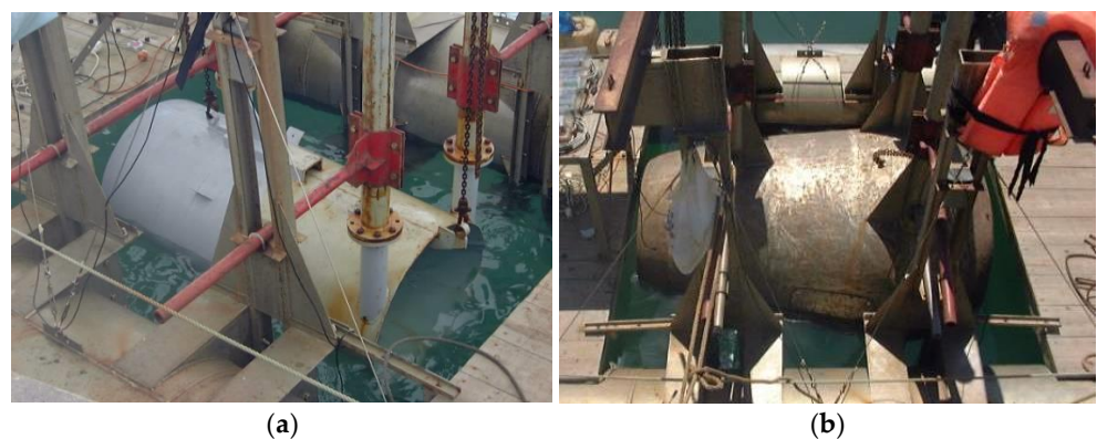
Figure 5. The duct scale models D2 (a) and D4 (b) at the higher level (partially immersed in the water) when the platform was tied to the quayside.
