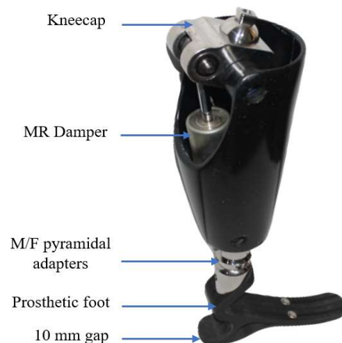
Figure 15. Rear view of the built prosthetic leg.
