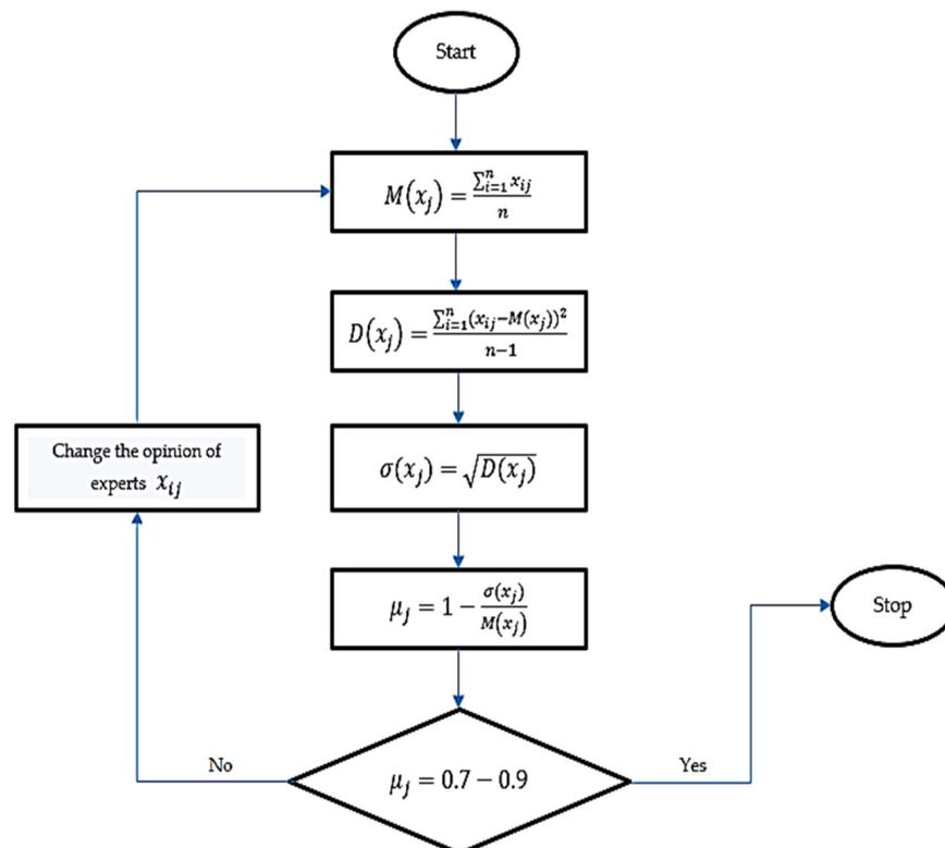
Figure 1. Flowchart of the process of the mean-square deviation method.
