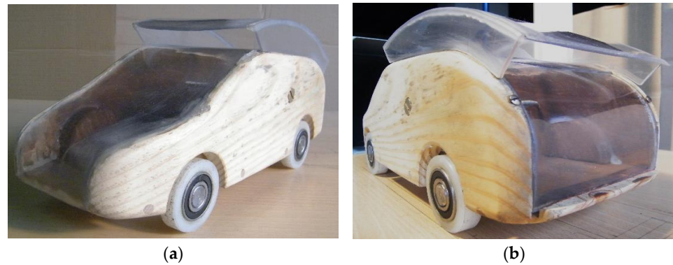
Figure 4. Car model with built-in deflector: (a) front side; (b) rear side.
