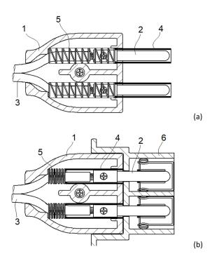
**Figure 1.** The utility model (**a**) represents a male plug when not connected. (**b**) represents the previous plug when inserted and connected to a base outlet.
