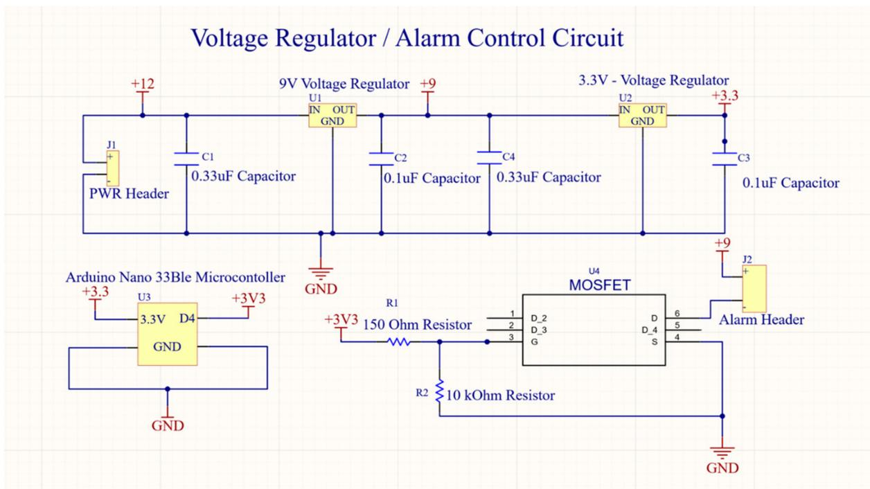
Figure 3. DiAtach alarm control circuit.
