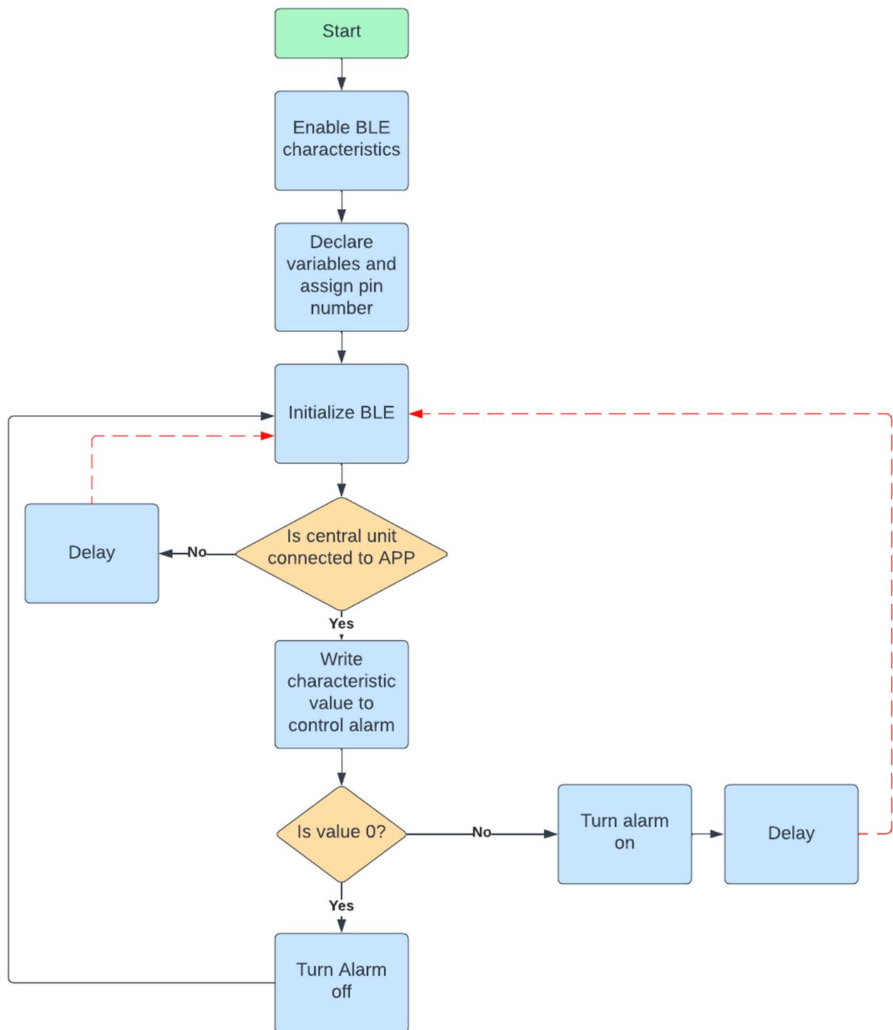
**Figure 6.** DiAttack Central Unit Software setting.
