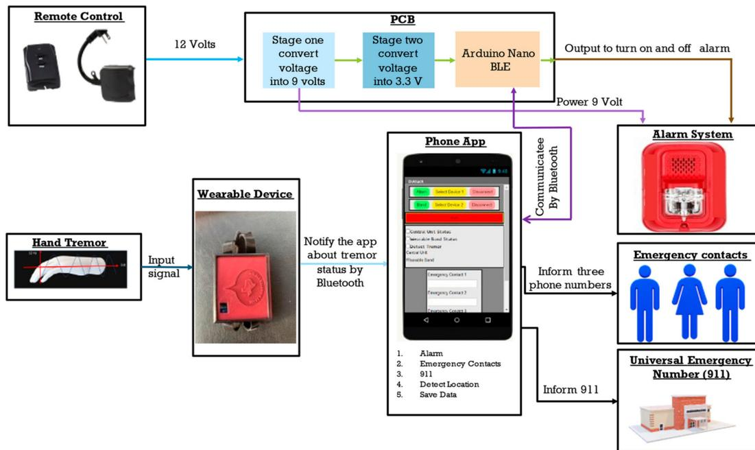
Figure 1. DiAttack Conceptual Block Diagram.
