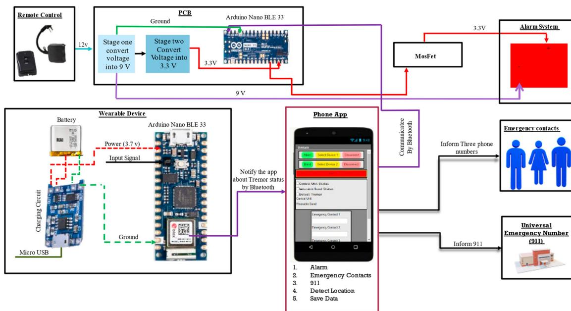
Figure 2. DiAttack functional block diagram.
