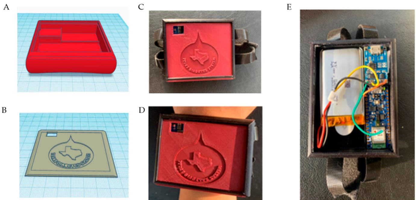
**Figure 8.** DiAttack wearable band. (A)—case, (B)—case cover, (C)—wearable device, (D)—wearing the wearable device and (E)—wearable device with its components.
