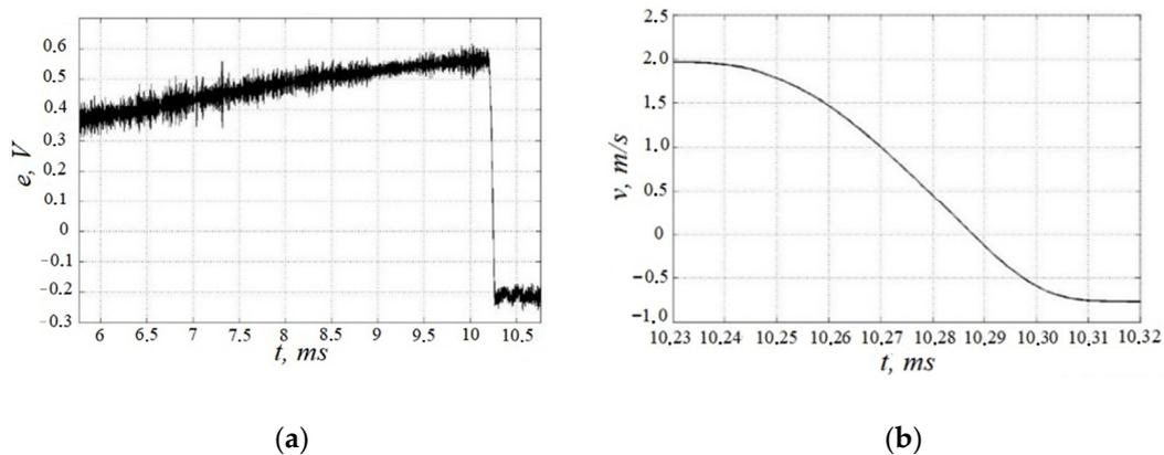
**Figure 6.** Graph of EMF  $e(t)$  induced on the induction coil during measurement (a) and graph of the impact body velocity during the indentation process (b).
