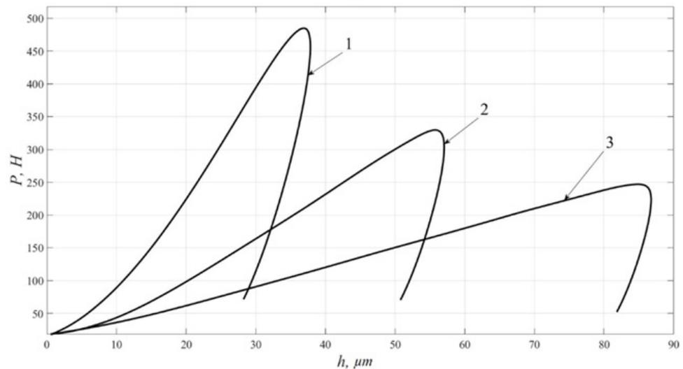
**Figure 9.** Load–displacement diagram curves for steel (1), brass (2) and aluminum (3) test blocks.
