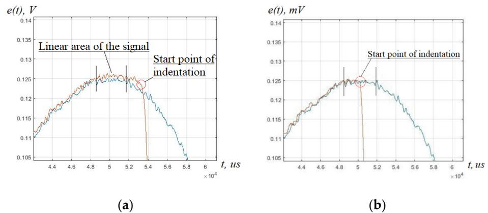
**Figure 5.** Signal obtained using a standardized (a) and modified (b) Leeb D impact device.
