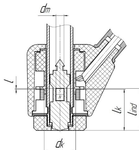
**Figure 3.** The location of the impact body relative to the induction coil at the time of indentation.
