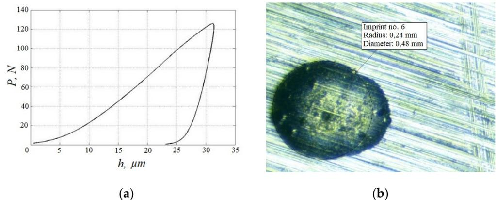
**Figure 8.** Load–displacement diagram (a) and photograph of the indentation (b).
