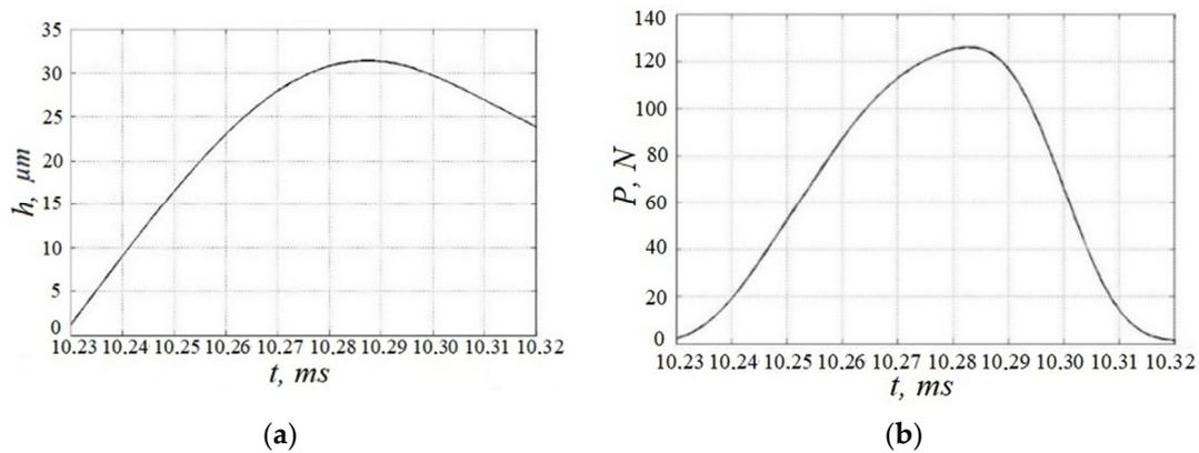
**Figure 7.** Graphs of the depth of penetration across time (a) and the graph of the applied load across time (b).
