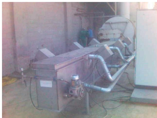
Figure 4. Pilot conveyor-belt dryer with tangential flow.
