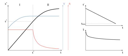
**Figure 1.** Schematic illustration of the charging and discharging behaviour of a lithium-ion battery. (**left**) Two-stage charging process plotted over time t. State of capacity  $s^+$  in black, voltage V in blue, and current A in red. (**top right**) State of capacity  $s^-$  during discharging over time t. (**bottom right**) State of capacity  $\bar{s}$  due to self-discharging.
