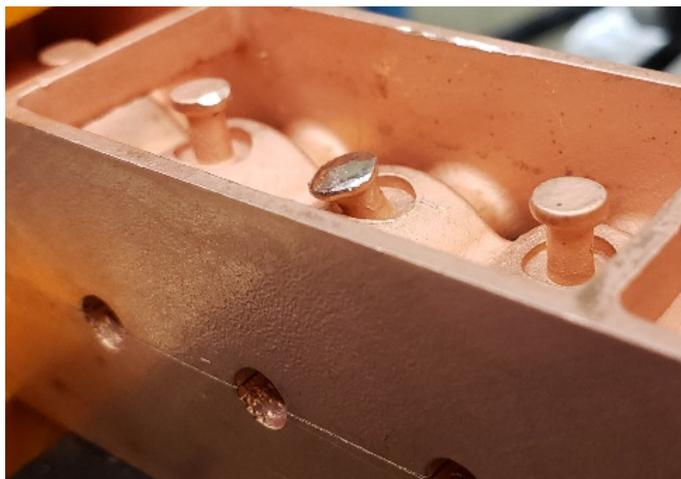
**Figure 15.** Deformed tuning pin after tuning test.
