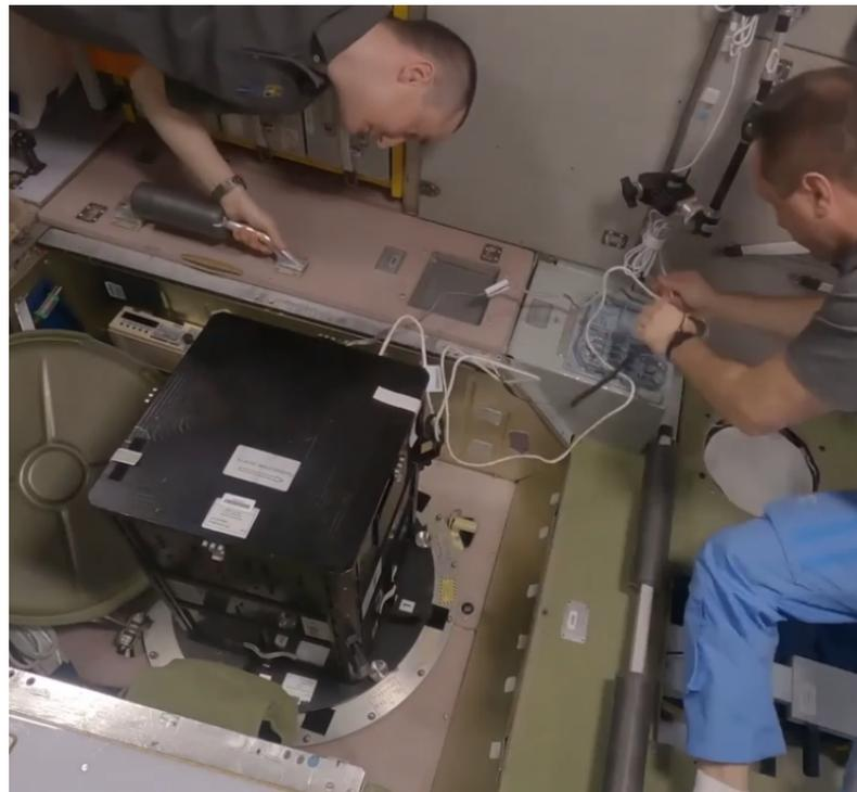
**Figure 3.** Mini-EUSO installed by two cosmonauts on the UV-transparent window of the Zvezda module.
